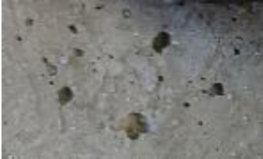
Figure 31: Bug holes seen on the surface of the 1.5% mixture specimen
