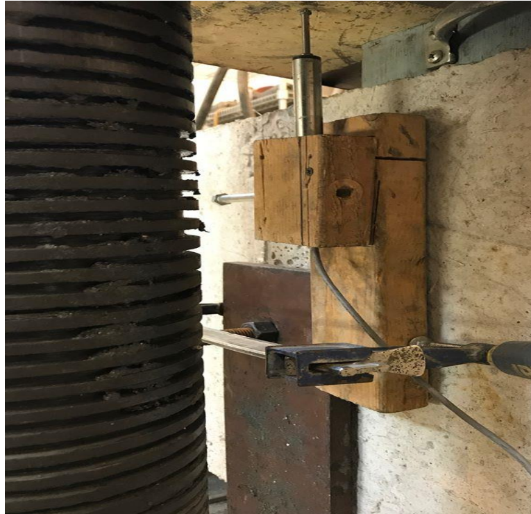
Figure18: Linear Variable Differential Transformers (LVDT) placement
