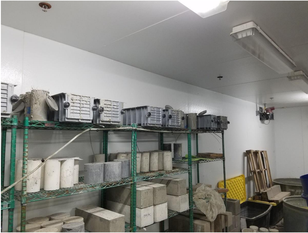
Figure 11: Small specimens placed inside curing room
