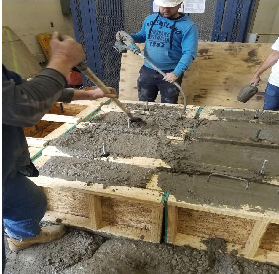
Figure 7: Concrete beam being vibrated and consolidated
