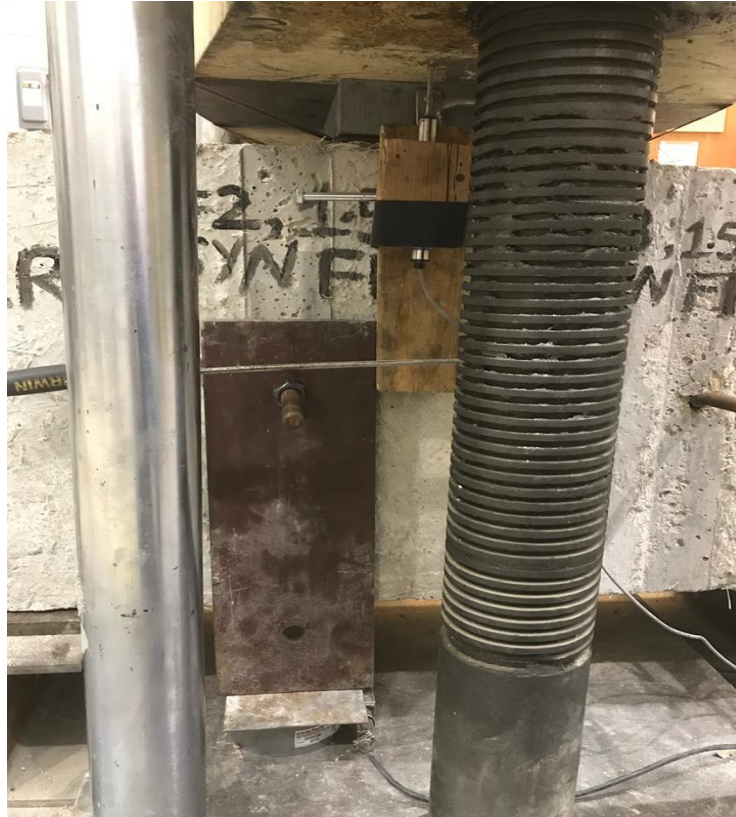
Figure17: Load cell placement
