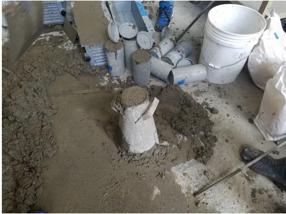
Figure 8: Filled slump cone
