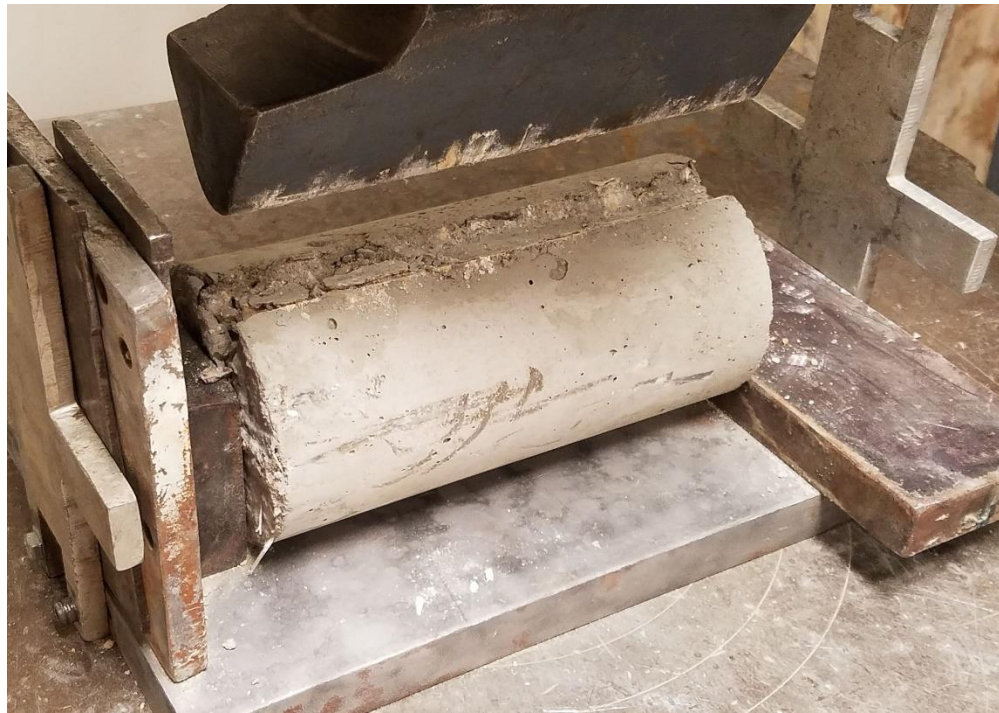
Figure 13: Split test setup
