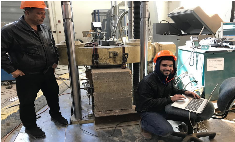
Figure 24: Shear test setup for anchors
