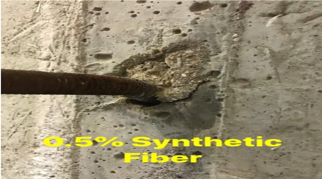
Figure 33: Steel failure preceded by concrete spall for 0.5% synthetic fiber
