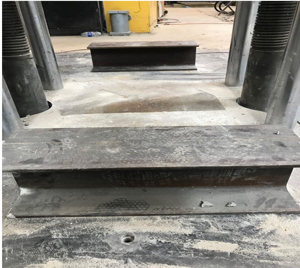
Figure15: Two "I" cross sectional steel members to support the specimen
