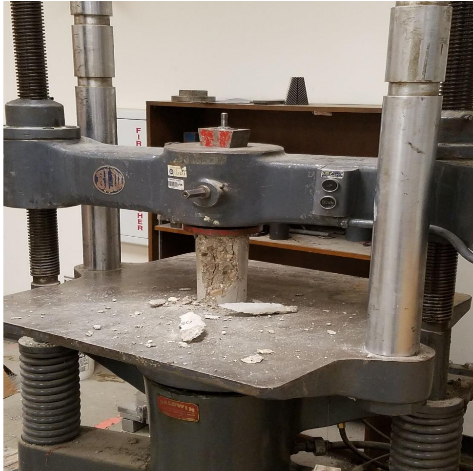
Figure 12: Compression Test Setup
