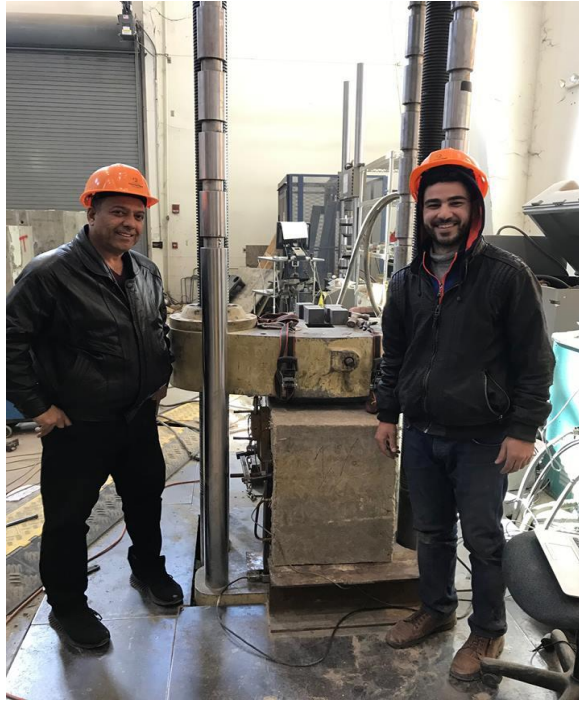
Figure 23: Shear test setup for anchors
