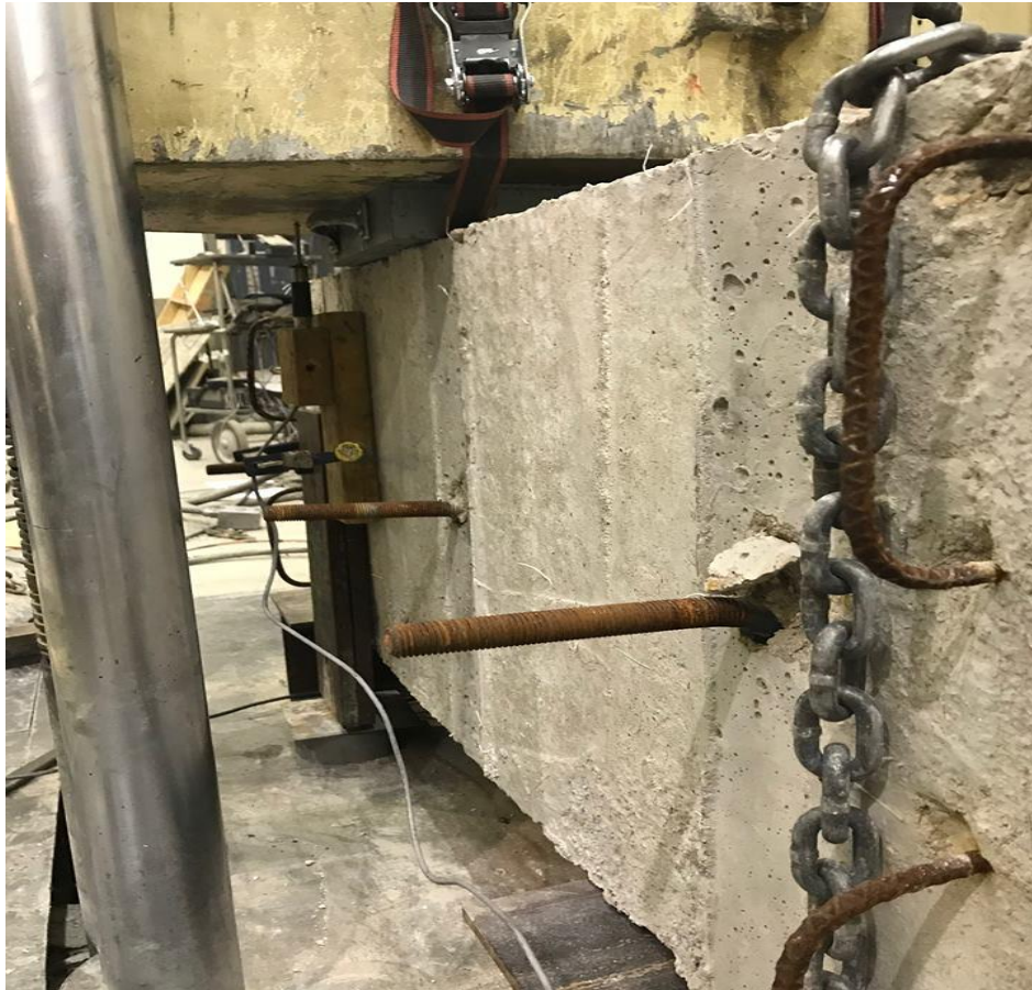
Figure 20: Applying different loading rate for the same specimen (0.50% Polypropylene Fiber)
