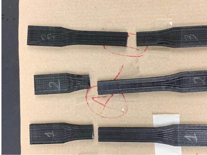
Figure 31: Fractured specimen of Stage-2
