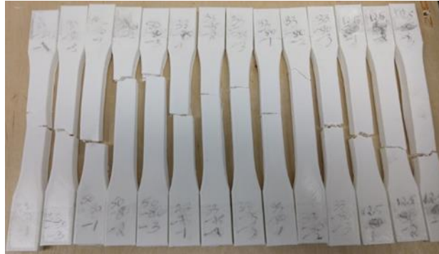
Figure 27:- Fractured set of specimens after mechanical testing for Stage-1
