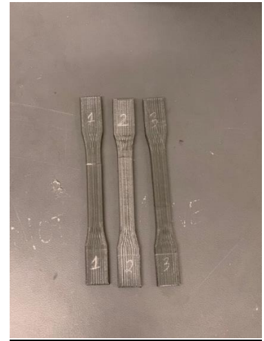
Figure 16: Stage-2 MTS specimens
