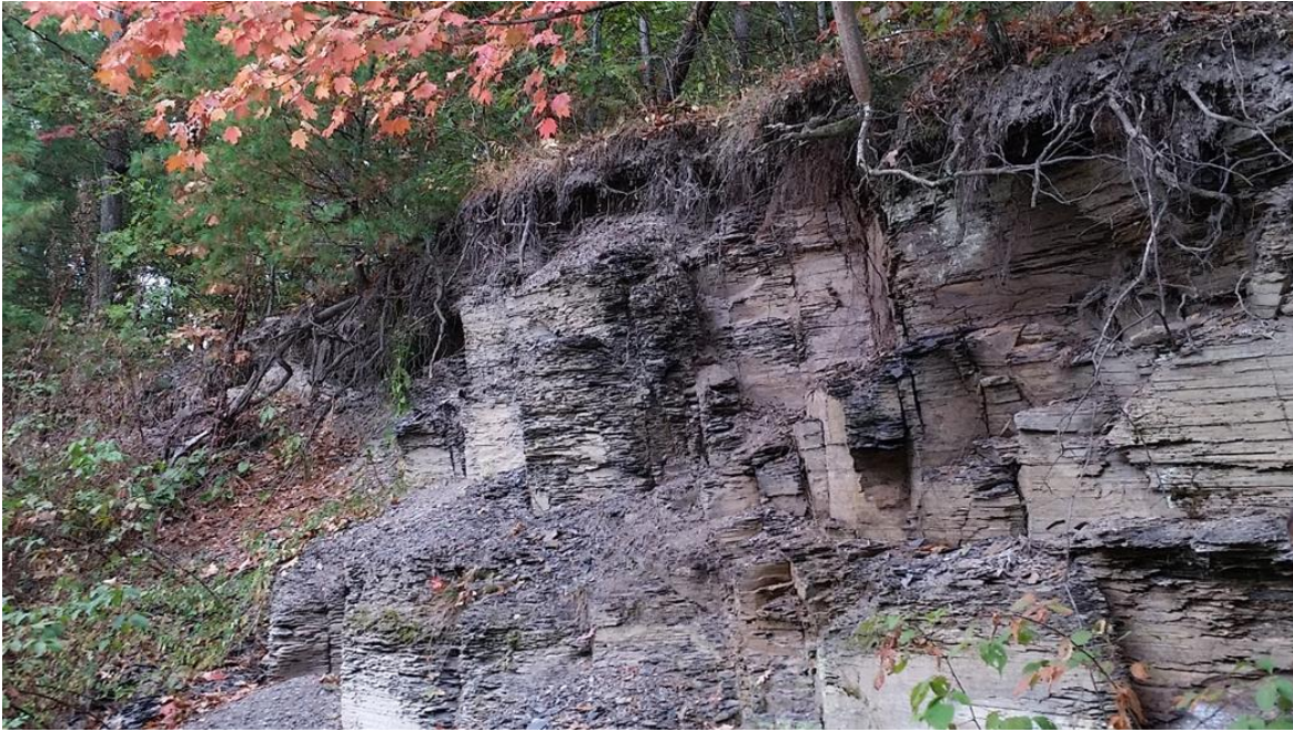
Figure 3-1: Hootenanny Camp Borrow Pit outcrop. Cold Springs Road, Huntingdon, PA. Shallow-dipping Marcellus Shale (Oatka Creek Member) revealing excellent jointing characteristics.
