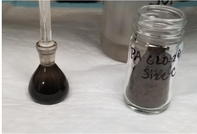
Figure 3-10: Pycnometer filled with CLO-240 size C sample plus DI water
