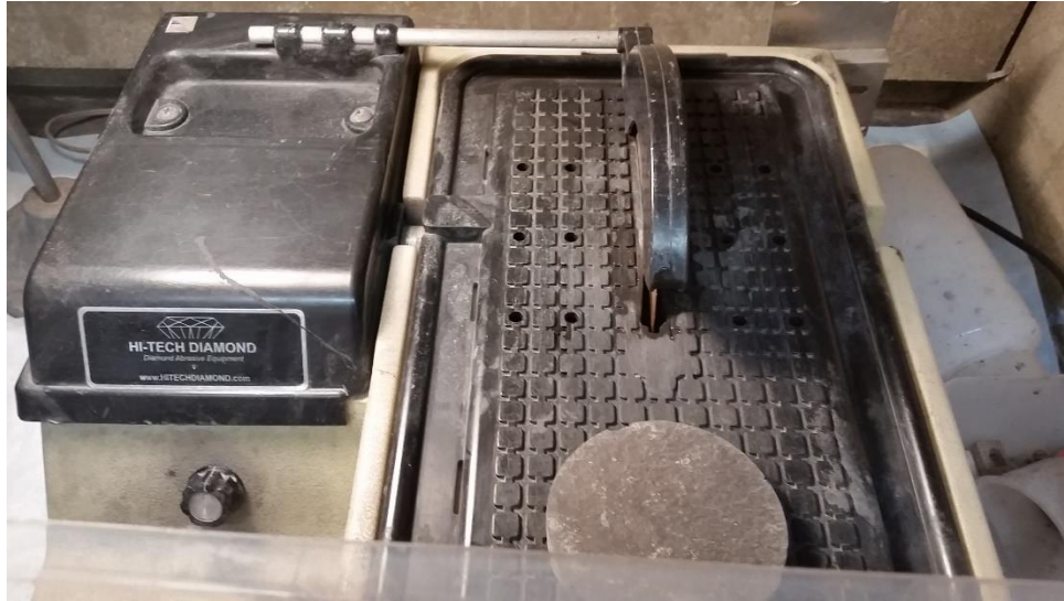
Figure 3-5: Hi-Tech Diamond saw used to cut samples into cubes.
