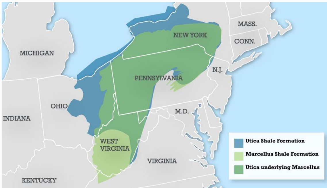
Figure 2-1: Boundaries of the Marcellus and Utica formations (from the Marcellus Shale Coalition, 2018).
