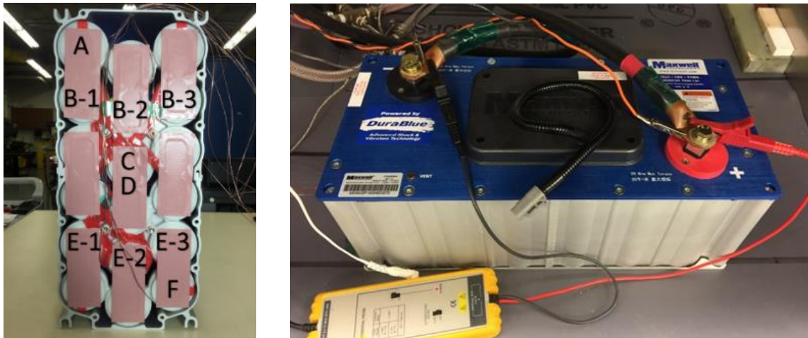
Figure 18: Maxwell 48 V module with the thermocouple placement (left) and the module inside the temperature chamber set up for testing.
