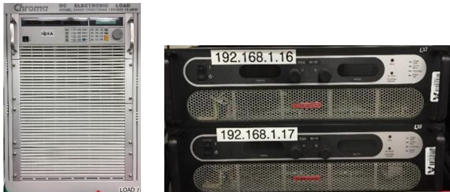
Figure 14: Photographs of the programmable load and supplies used to cycle the cells and modules for this experiment.
