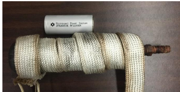
Figure 88: Pipe housing, heat tape, and LiFePO 4 cell setup used to direct vented gas into the acrylic test chamber.
