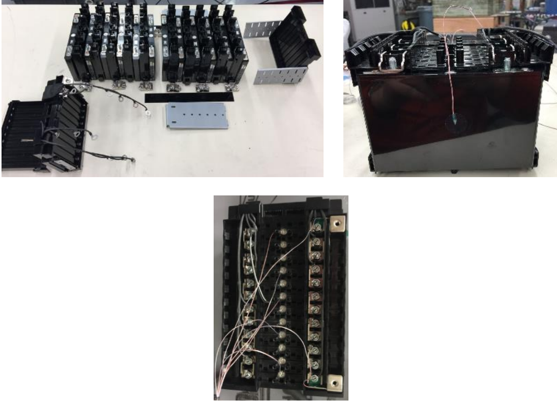
Figure 20: JM Energy 45 V module fully disassembled (left) to place thermocouples of the body of multiple cells (center). The module with multiple cells instrumented and reassembled (right).
