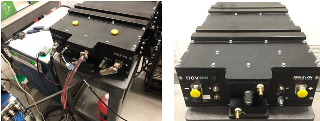
Figure 23: Skeleton 170 V module sitting in an ambient environment, being cycled.
