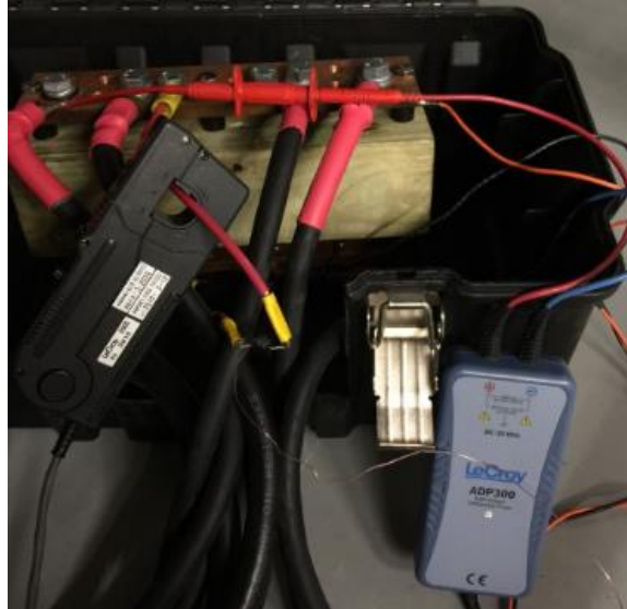
Figure 59: The system setup using the 15KPA33CA, differential voltage probes, and current meter.
