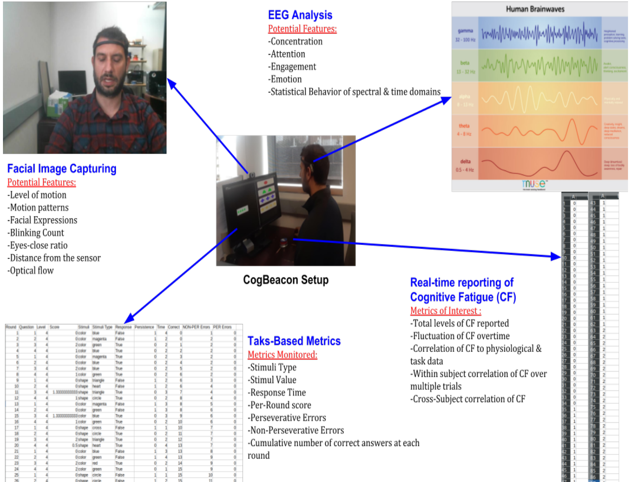
Figure 6.11. The CogBeacon Data Collection Framework. CogBeacon is an open-access software 5 . It currently supports multiple variations of the WCST cognitive task and in future versions will be enriched with additional cognitive games. It is easy to download and install almost in any platform and can easily support the integration of different sensing devices. Currently, data have been collected using a single RGB web-camera and the MUSE EEG headset. However, integrating additional sensor is very intuitive as long as they have an API that listens to Python programming language.
