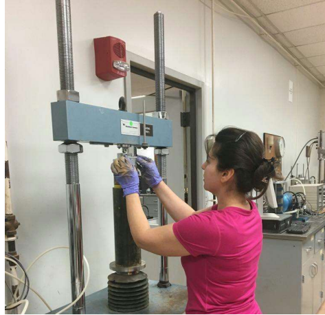
Figure 3-6 Compaction of the permeability test sample
