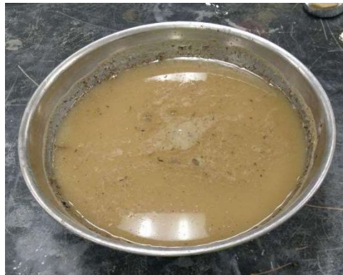
Figure 3-8 Soil sample soaked in water for 24 hours
