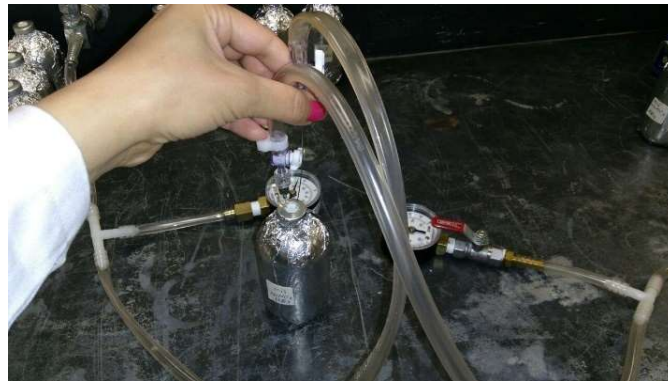
Figure 3-18 Pressure and vacuum gauge to control the flushing process
