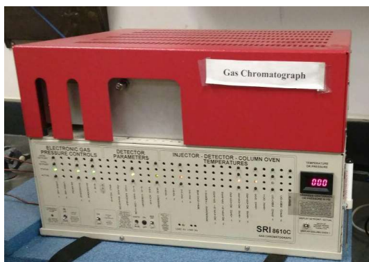
Figure 3-20 Gas chromatograph (GC, SRI 8610)
