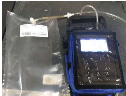
Figure 3-30 Tedlar bag connected to Landtec hydrogen sulfide analyzer
