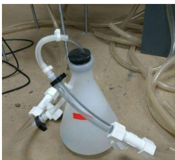
Figure 3-26 Humidifier connected to the gas cylinder and column
