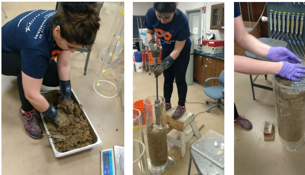
Figure 3-22 The process of mixing and compacting soil inside the column
