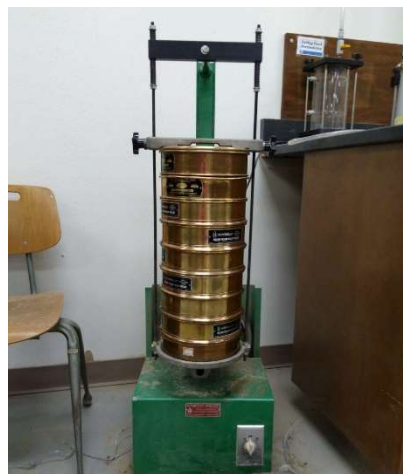
Figure 3-10 Sieve shaker and sieve stack for the sieve analysis
