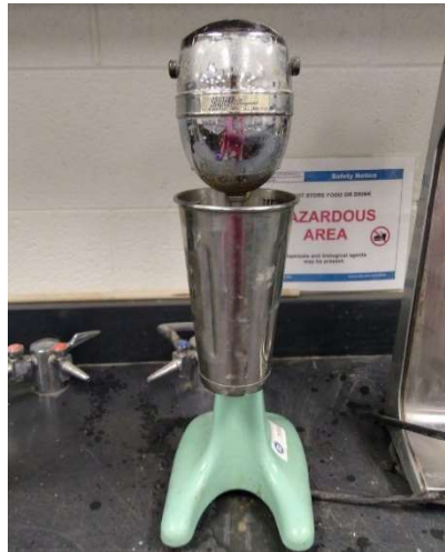
Figure 3-12 Process of mixing the sample before the hydrometer test
