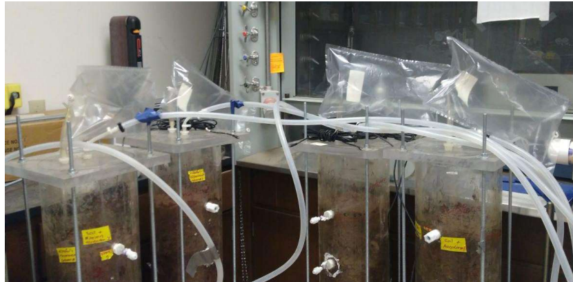
Figure 3-29 Collecting gas samples from the surface of the soil for gas analysis
