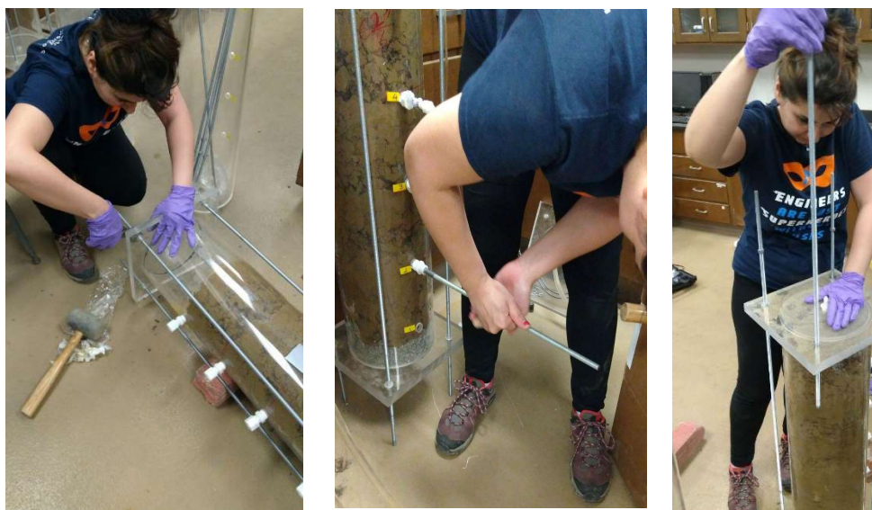
Figure 3-23 The process of setting up the first column reactor
