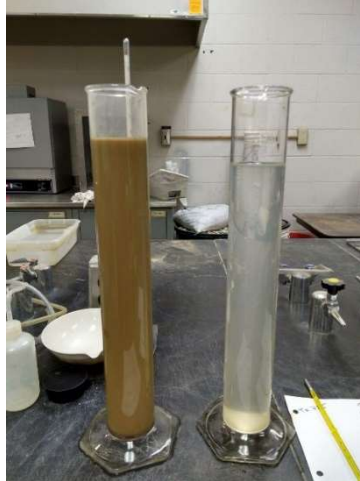
Figure 3-13 Hydrometer test setup
