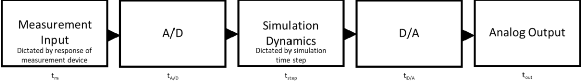
Figure 7. Delay that is experienced during a PHIL deployed generation source [8].
