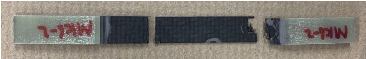
Figure 30: Fatigue failure of Paper structural Capacitor coupon
