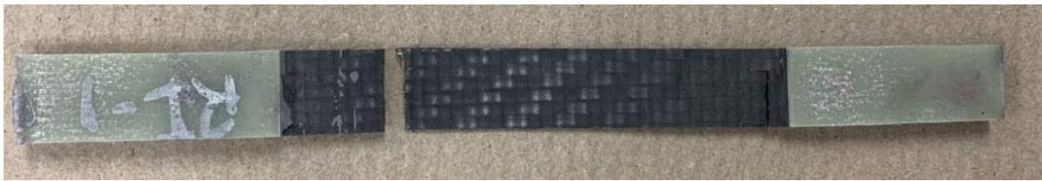
Figure 27: Fatigue Failure of 4Ply Carbon Fiber coupon
