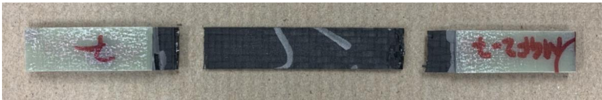
Figure 24: Fatigue failure of Glass Fiber structural Capacitor coupon
