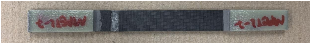
Figure 28: Fatigue failure of PET structural Capacitor coupon
