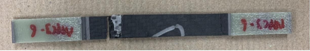
Figure 25: Fatigue failure of PC structural Capacitor coupon
