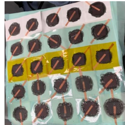
Figure 12: 2"x2" samples for capacitance measurement
