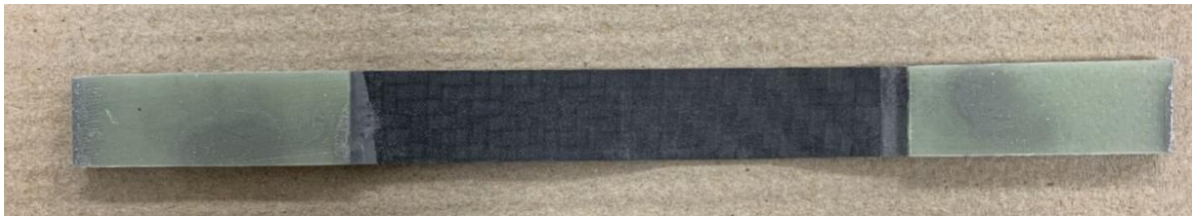
Figure 17: Sample for Fatigue and Tensile testing
