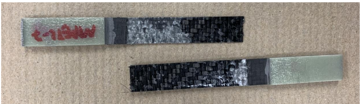
Figure 29: Fatigue failure of PET structural Capacitor coupon due to delamination in PET and electrode interface
