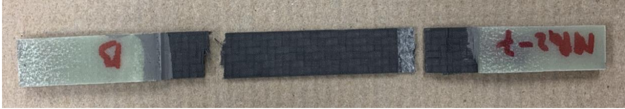
Figure 30: Fatigue failure of Paper structural Capacitor coupon
