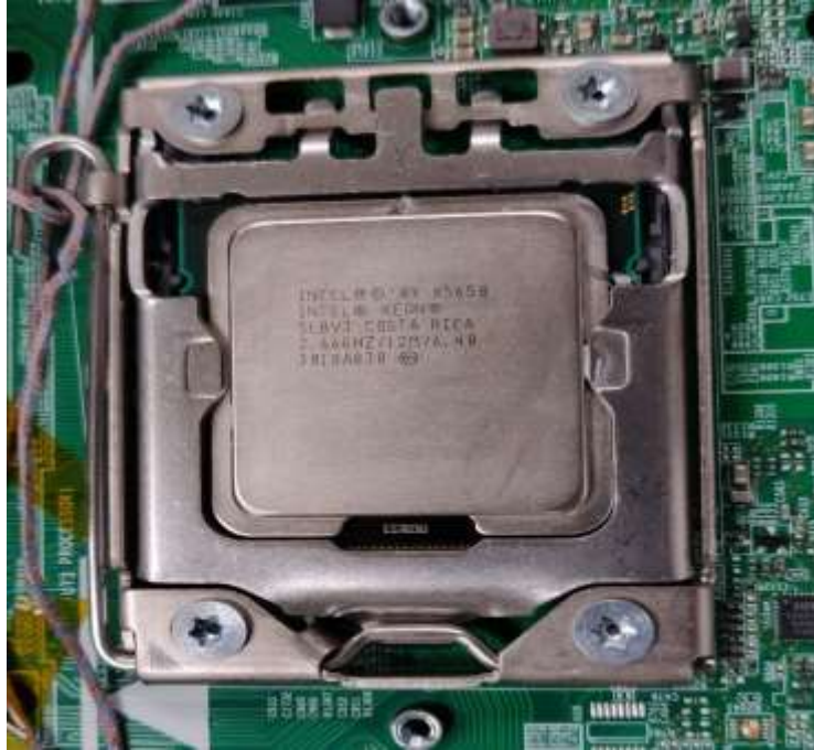
Figure 25: CPU Processor without the TIM
