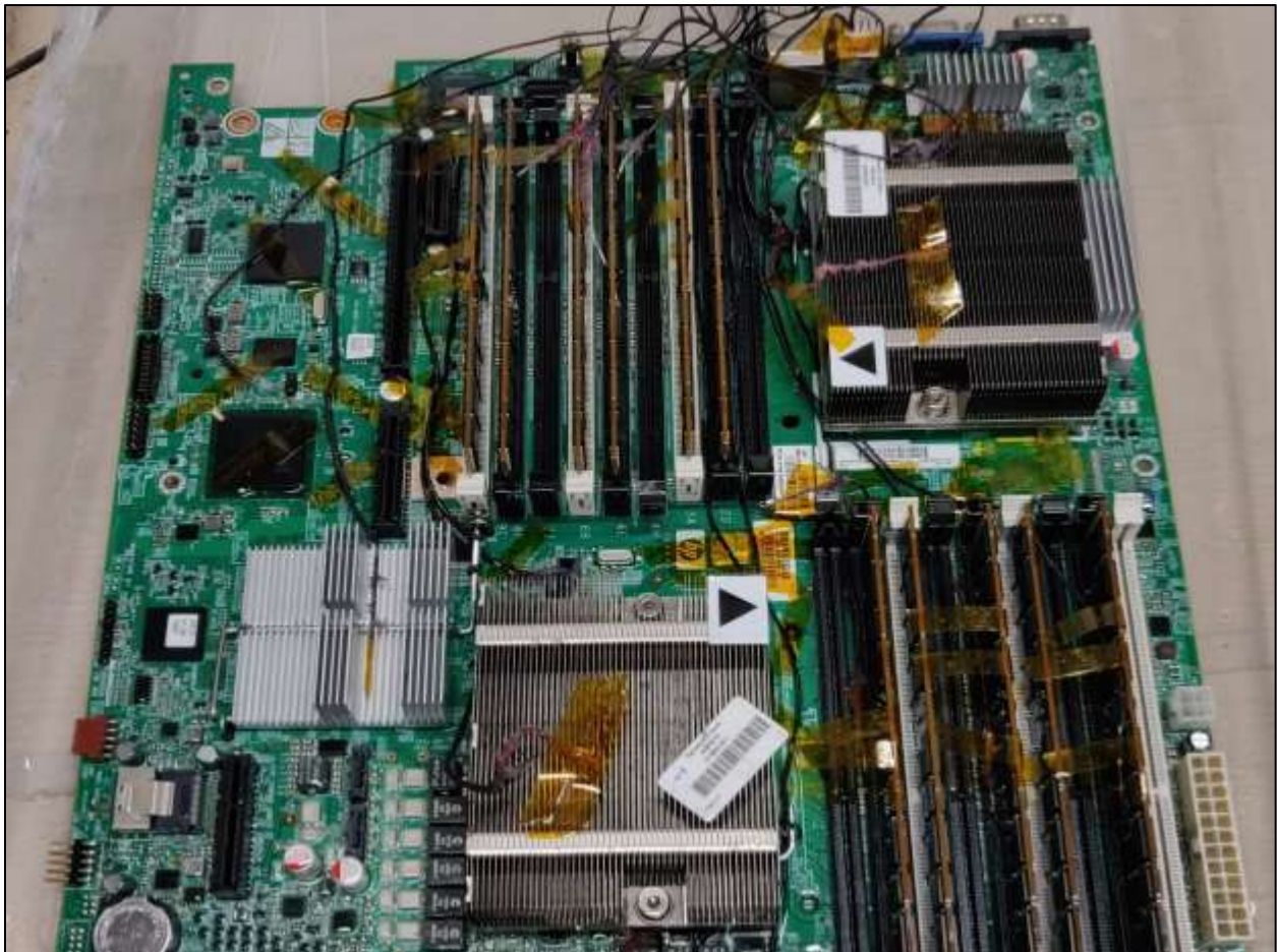
Figure 11: Thermocouple Connections in the Server
