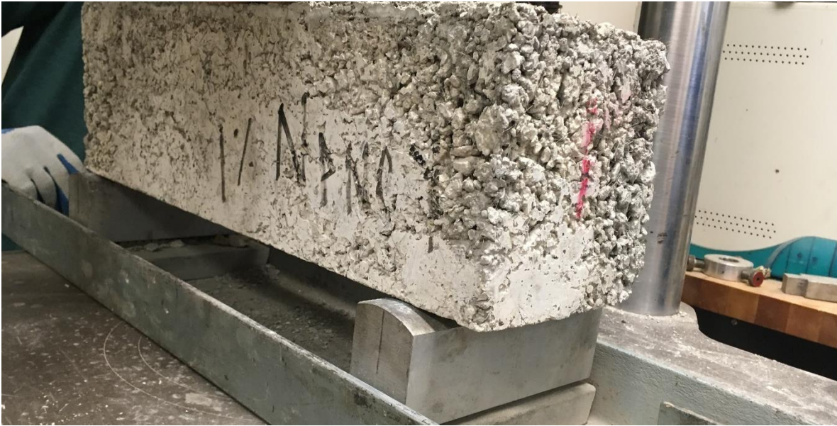
Figure 36. 1% SFRC Beam-Modulus of Rupture Test Setup
