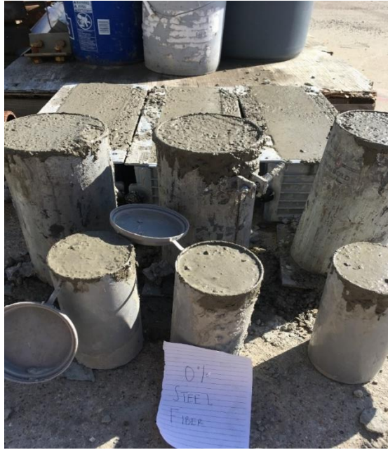
Figure 11. 0% SFRC in Beam and Cylinder Molds
