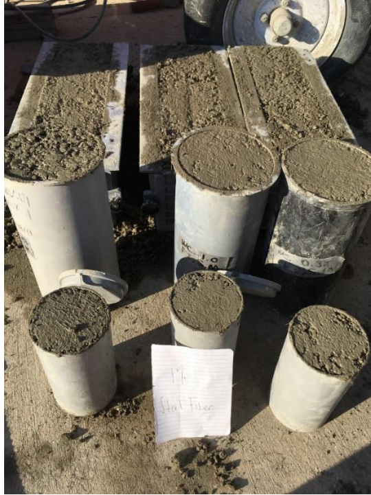
Figure 13. 1% SFRC Batch in Beam and Cylinder Molds
