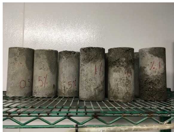
Figure 16. 4" x 8" Cylinders for Compression Test
