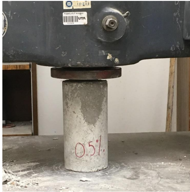
Figure 26. 0.5% Cylinder (4" x 8") Compression Test Setup
