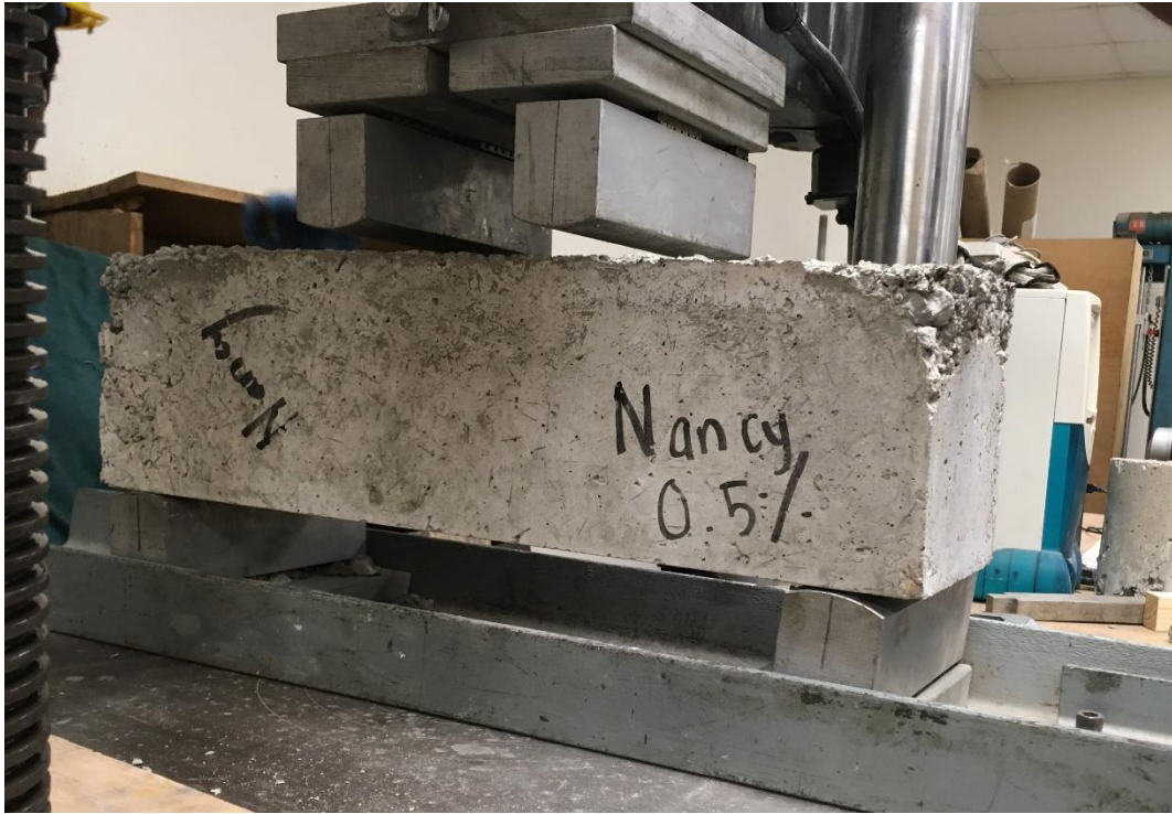
Figure 34 0.5% SFRC Beam-Modulus of Rupture Setup
