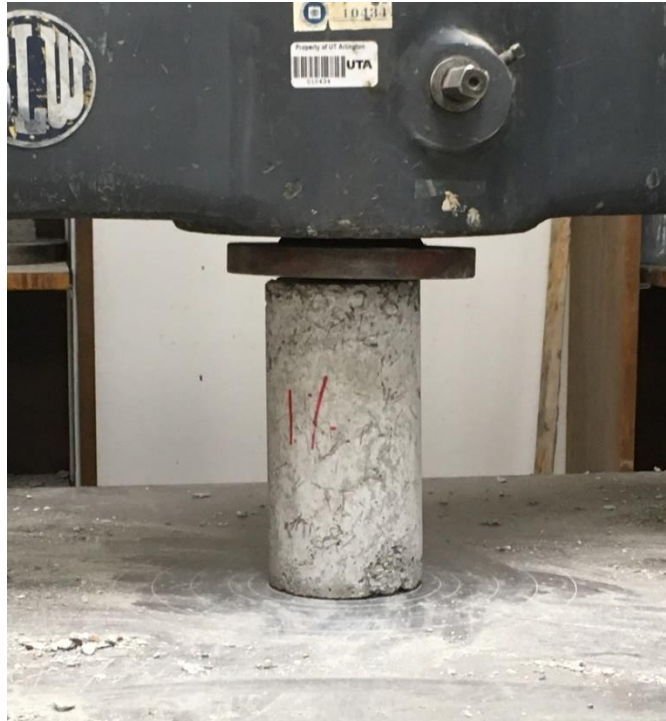
Figure 28. 0.5% Cylinder (4" x 8") Compression Test Setup
