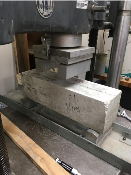
Figure 32. 0% SFRC Beam-Modulus of Rupture Setup
