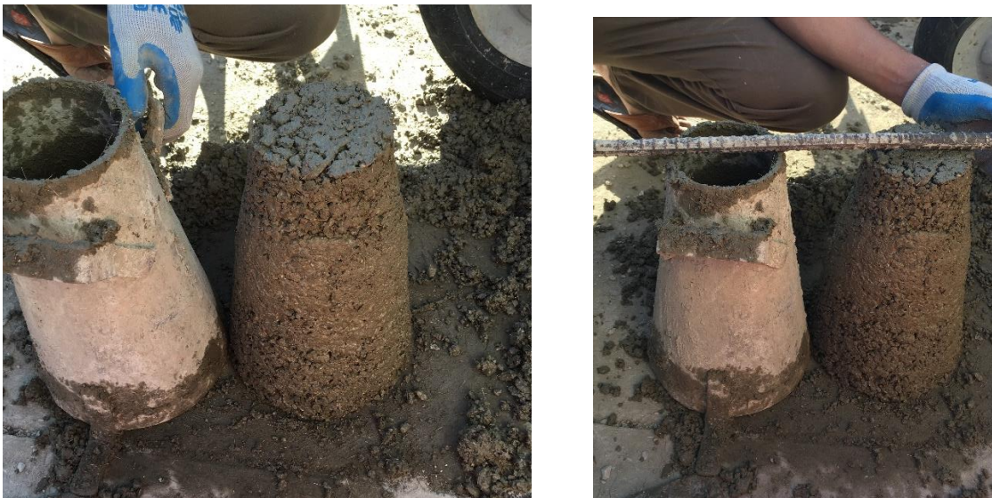
Figure 14. Slump Test on 0.5% Concrete Mix
