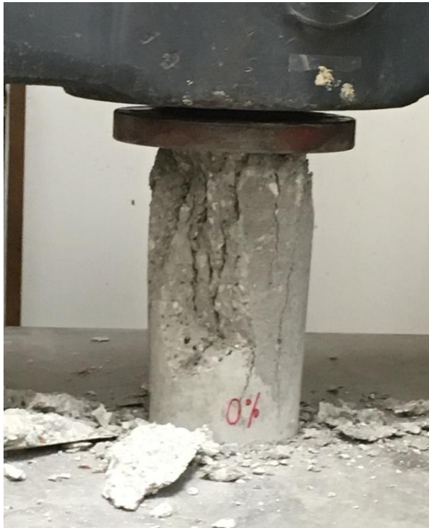
Figure 25. 0% Cylinder collapses at 36 kips
