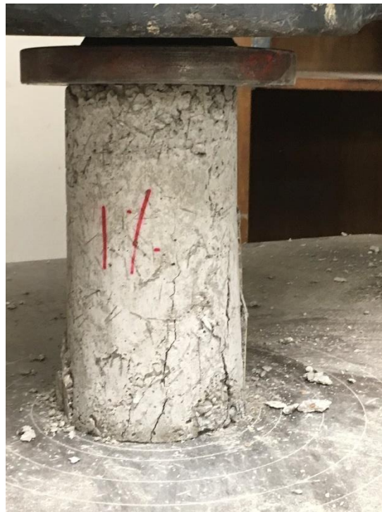
Figure 29. 1% Cylinder collapses at 53 kips
