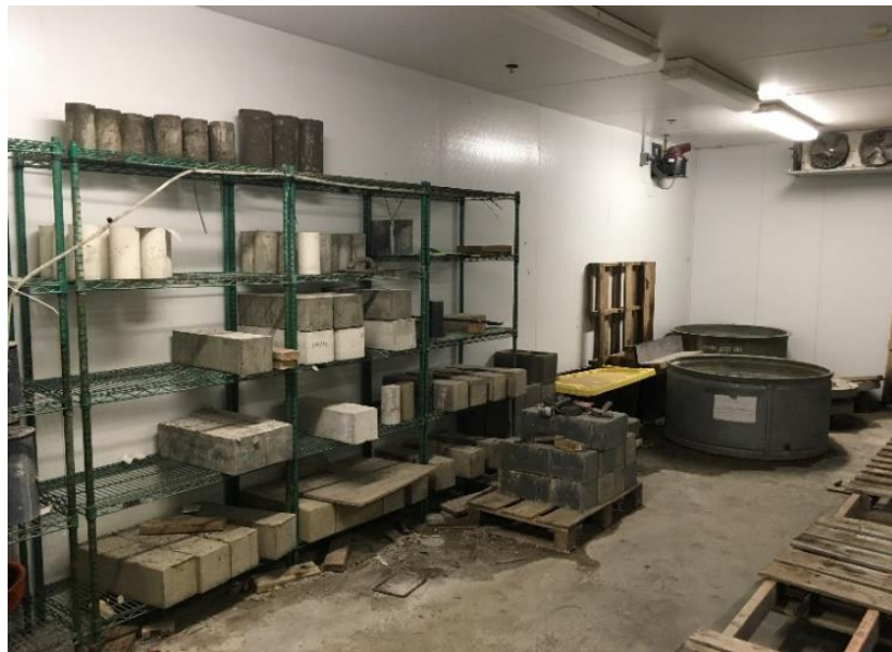
Figure 15. Humidity Controlled Room
