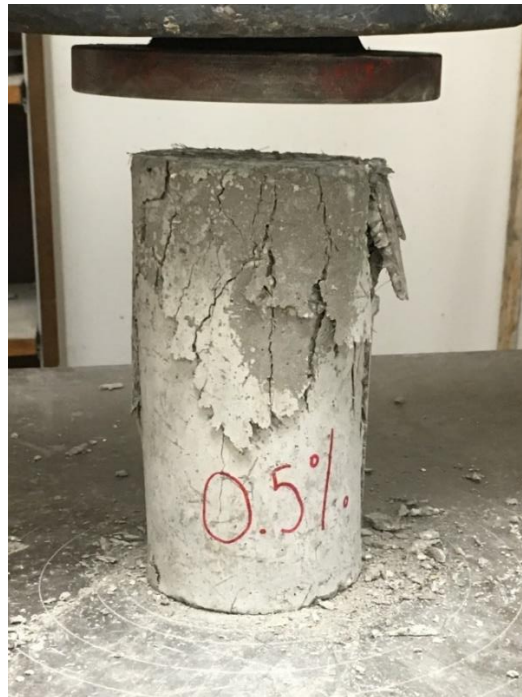
Figure 27. 0.5% Cylinder collapses at 48 kips
