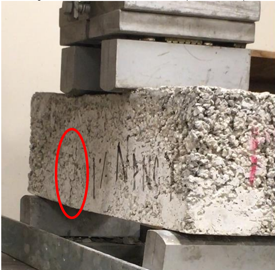
Figure 37. 1% SFRC Beam at Failure Load is 8.7 kips
