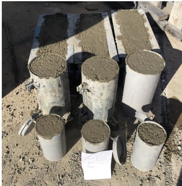
Figure 12. 0.5% SFRC in Beam and Cylinder Molds
