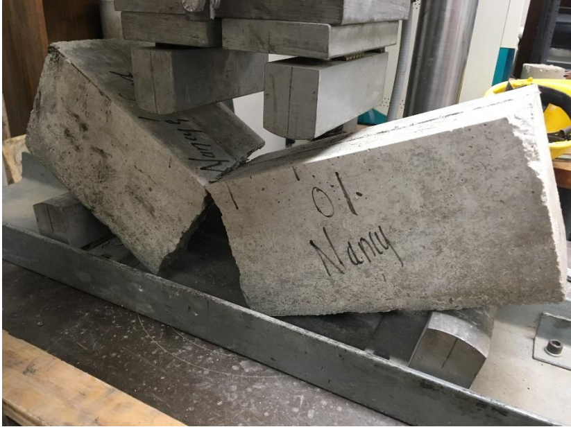
Figure 33. 0% SFRC Beam at Failure Load 6.6 kips
