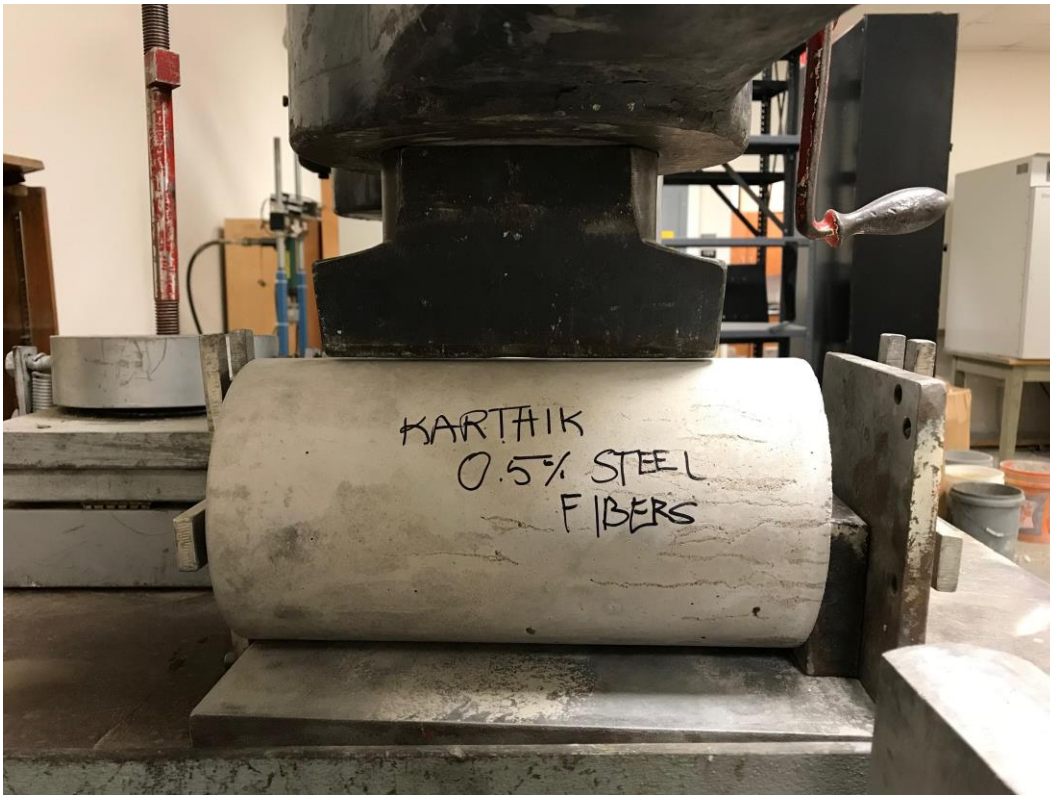
Figure 21 Split tensile test of concrete cylinder of 0.5% steel fiber by volume
