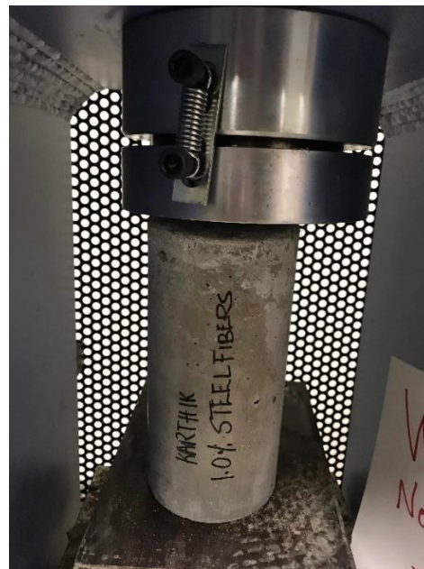
Figure 20 Compression test of concrete for 1% steel fiber by volume before test.
