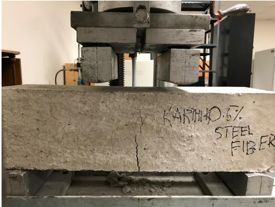
Figure 23 Modulus of rupture test of concrete beam of 0.5% steel fiber by volume
