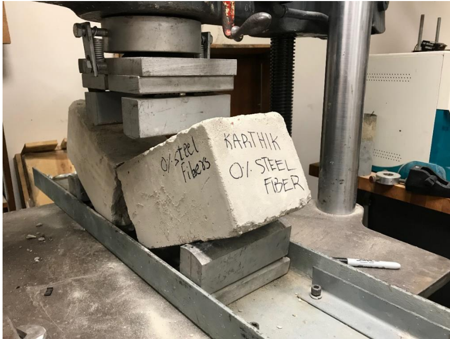
Figure 22 Modulus of rupture test of concrete beam of 0.0% steel fiber by volume
