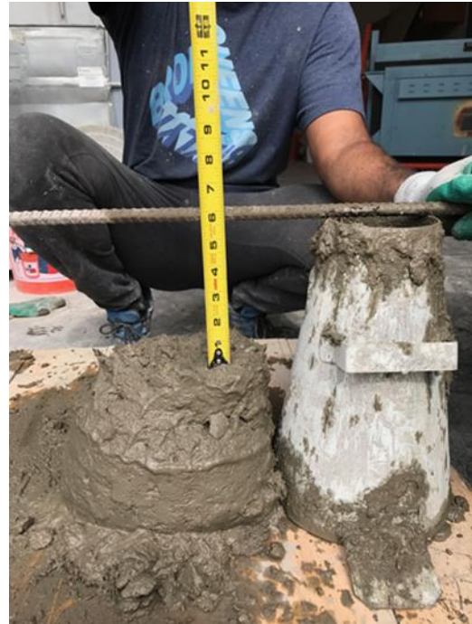
Figure 12 Slump test of 0.5% steel fiber reinforced concrete
