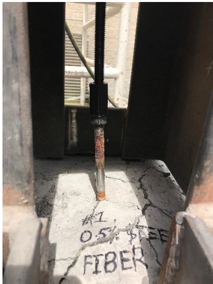
Figure 26 0.5% steel fiber reinforced concrete beam with embedded anchor bolt.
