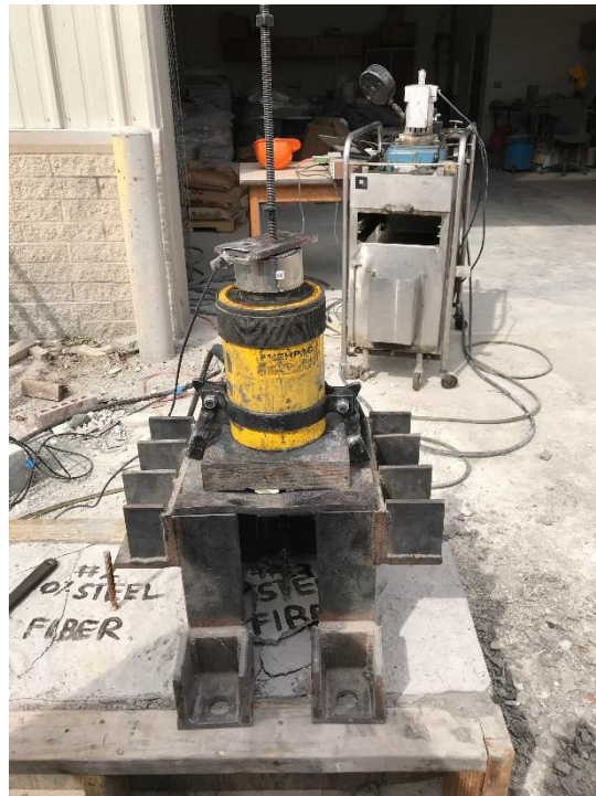
Figure 14 Test set-up, frame, hydraulic ram and load cell
