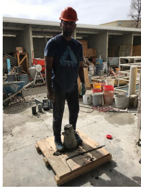
Figure 9 Slump cone procedure
