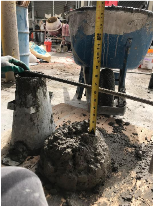
Figure 11 Slump test of 0.0% steel fiber reinforced concrete
