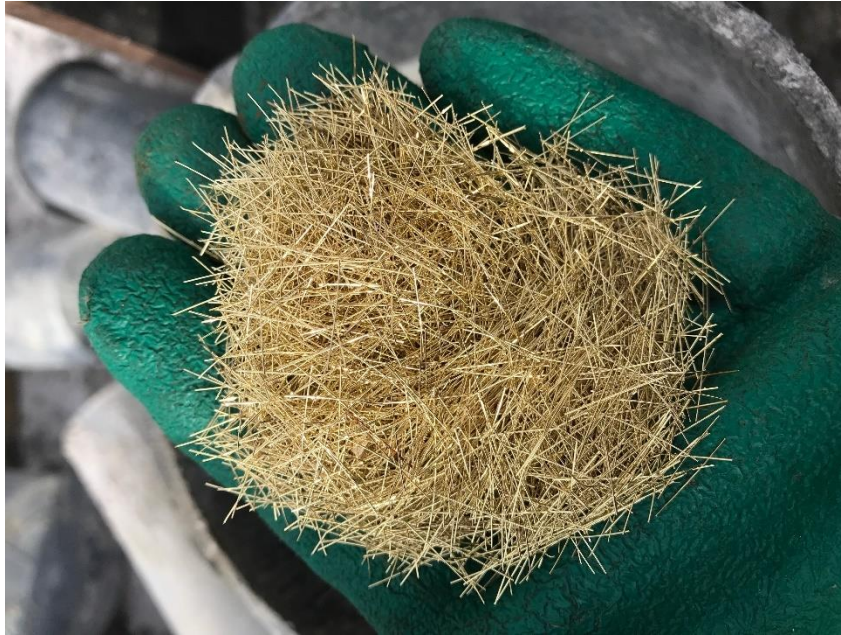
Figure 3 Steel fibers used in this research
