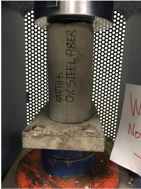
Figure 17 Compression test of concrete for 0% steel fiber by volume before test.
