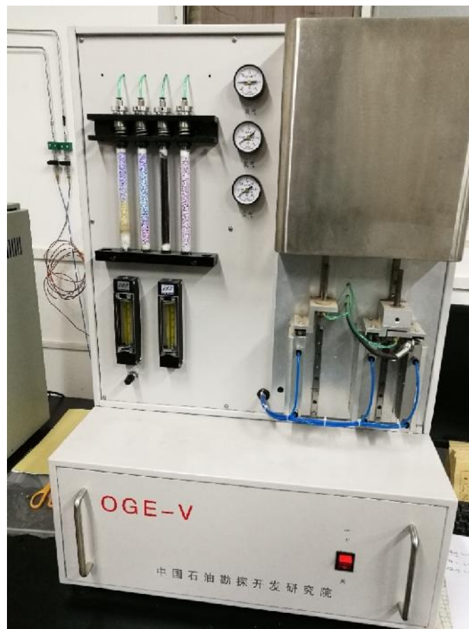
Figure 7. Pyrolysis analyzer of OGE-V Oil and Gas Evaluation Station.
