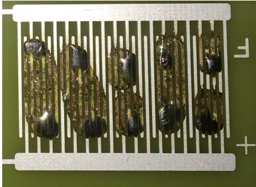
Figure 6-6 Corrosion due to the conducting nature of the NaCl salt solution at a relative humidity higher than the DRH.
