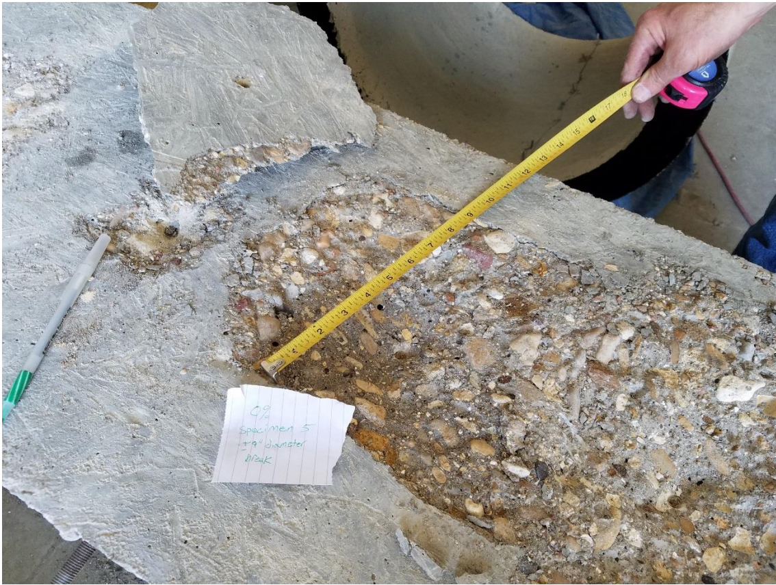
Figure 36: 0.0% Fiber - Specimen 5 Failure
