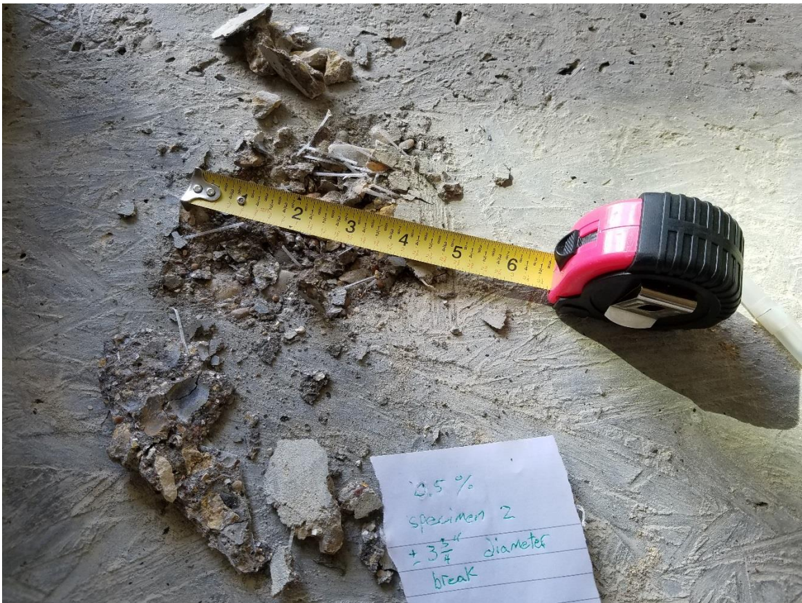
Figure 38: 0.5% Fiber - Specimen 2 Failure
