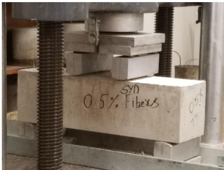
Figure 12: Flexure Test Setup
