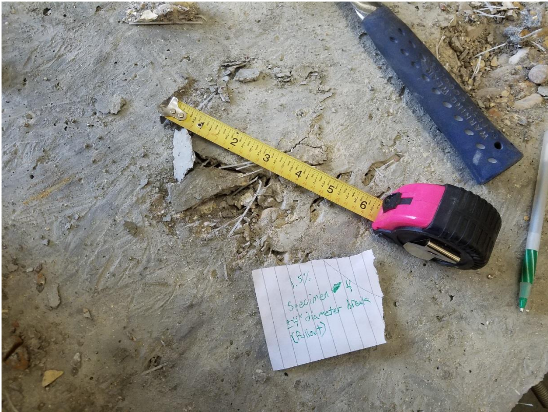
Figure 50: 1.5% Fiber - Specimen 4 Failure
