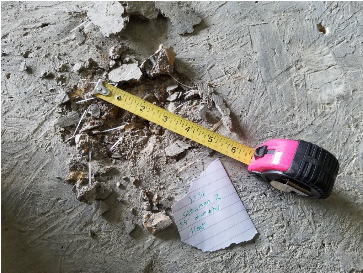
Figure 43: 1.0% Fiber - Specimen 2 Failure
