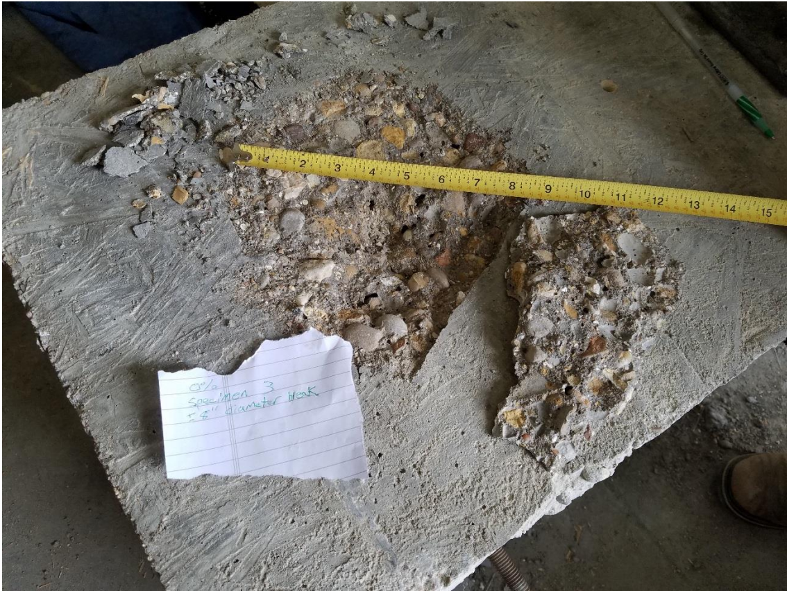
Figure 34: 0.0% Fiber - Specimen 3 Failure
