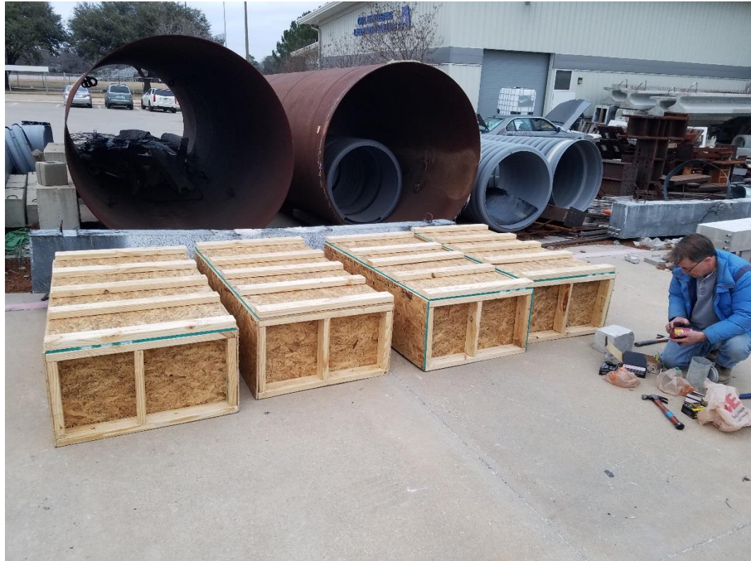
Figure 4: Wood Frames for Anchor Specimens
