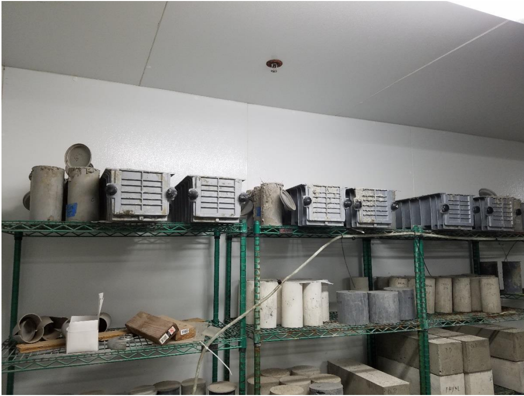
Figure 9: Small specimens placed inside curing room
