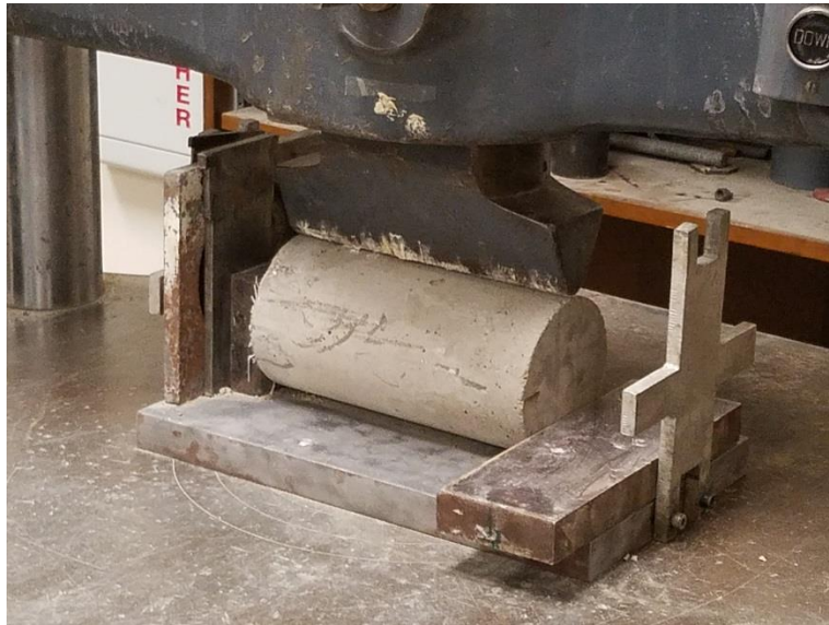
Figure 11: Split Test Setup
