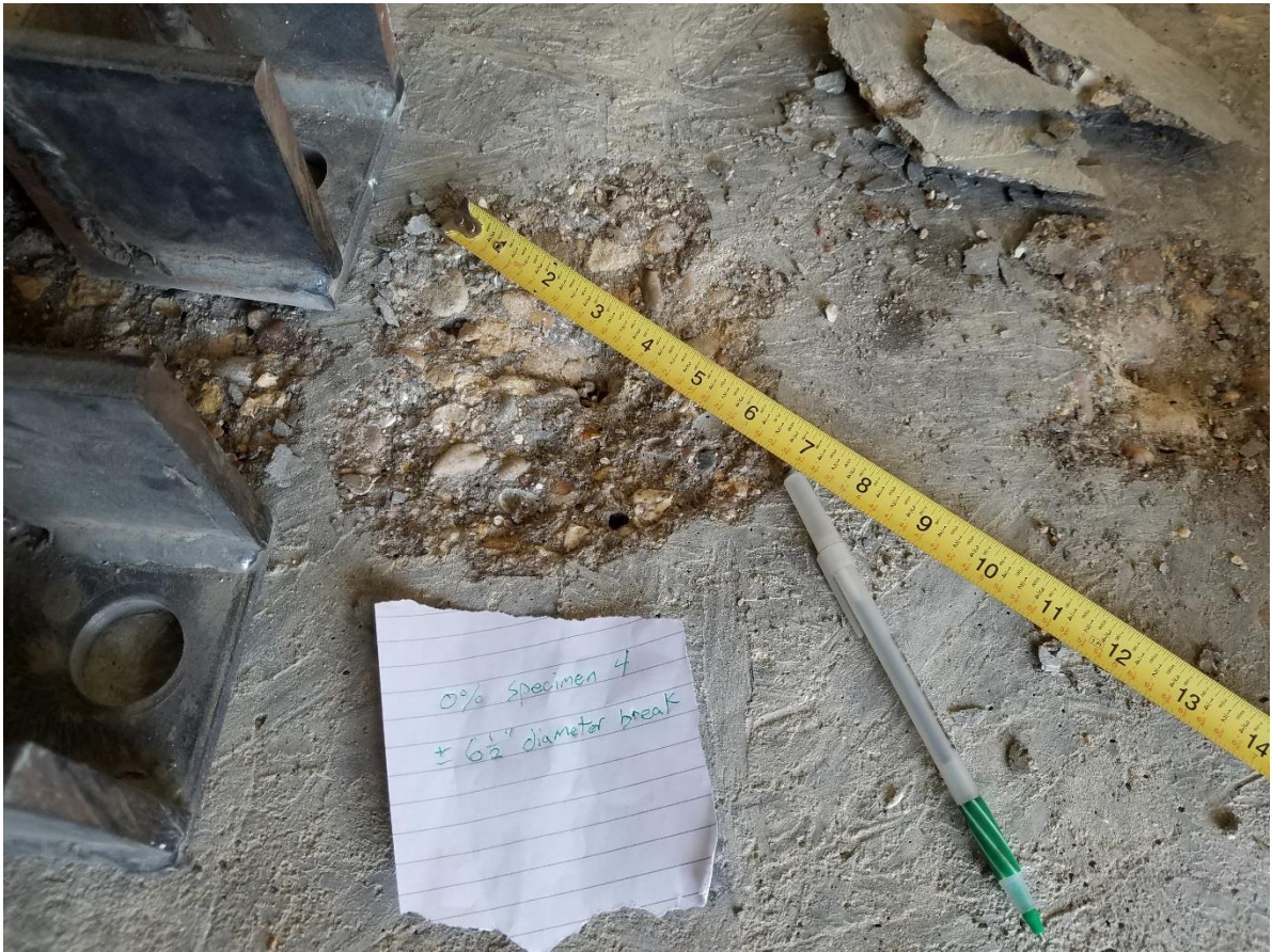
Figure 35: 0.0% Fiber - Specimen 4 Failure
