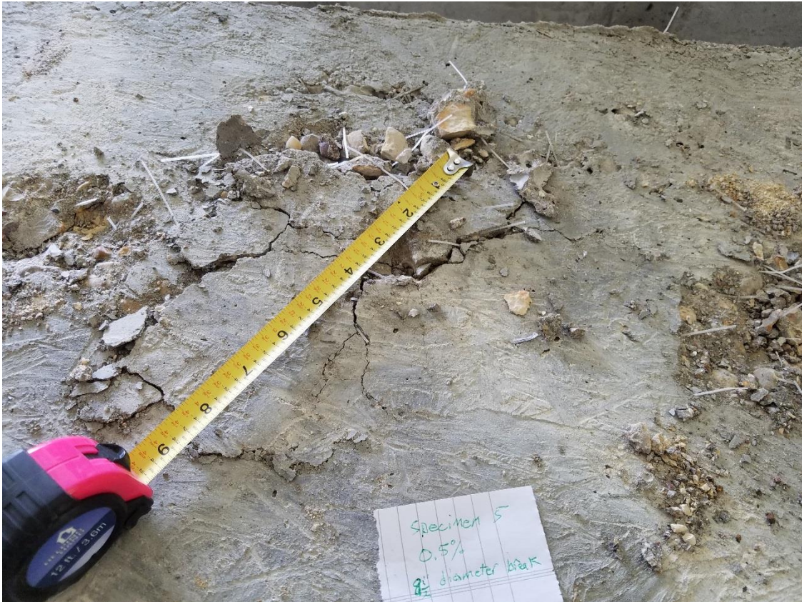
Figure 41: 0.5% Fiber - Specimen 5 Failure
