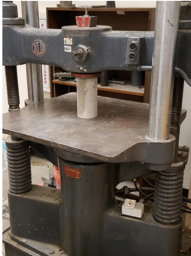
Figure 10: Compression Test Setup
