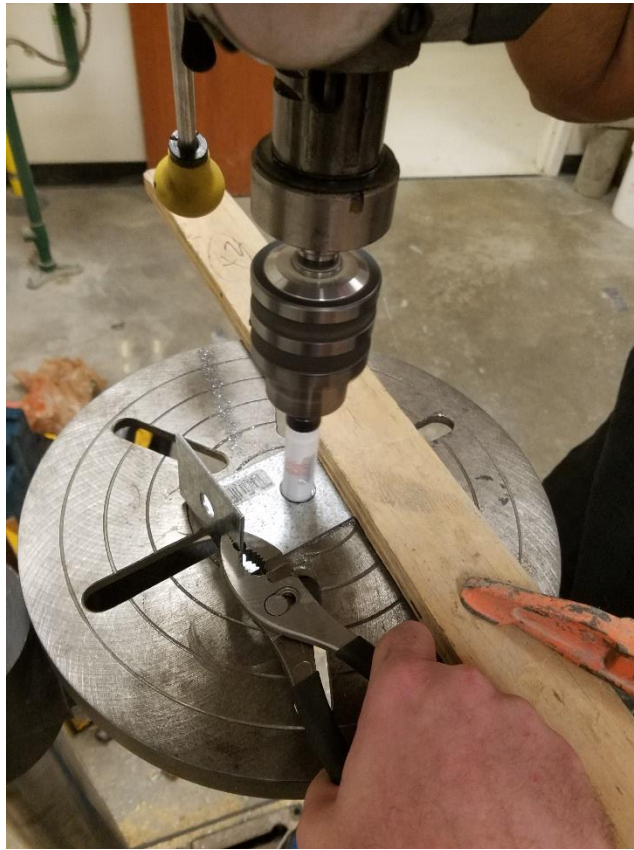
Figure 13: Holes are drilled into steel angles as needed for the testing setup
