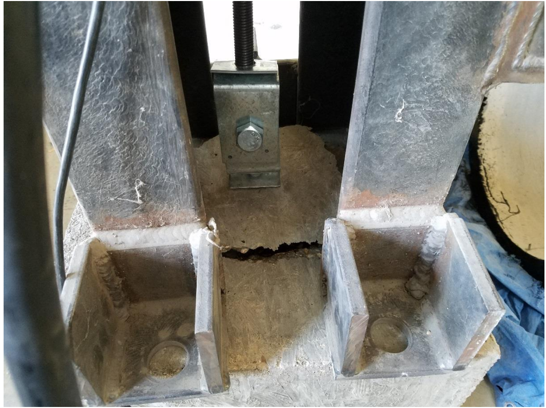
Figure 19: Specimen 1 of the 0.0% fiber beam breaking out
