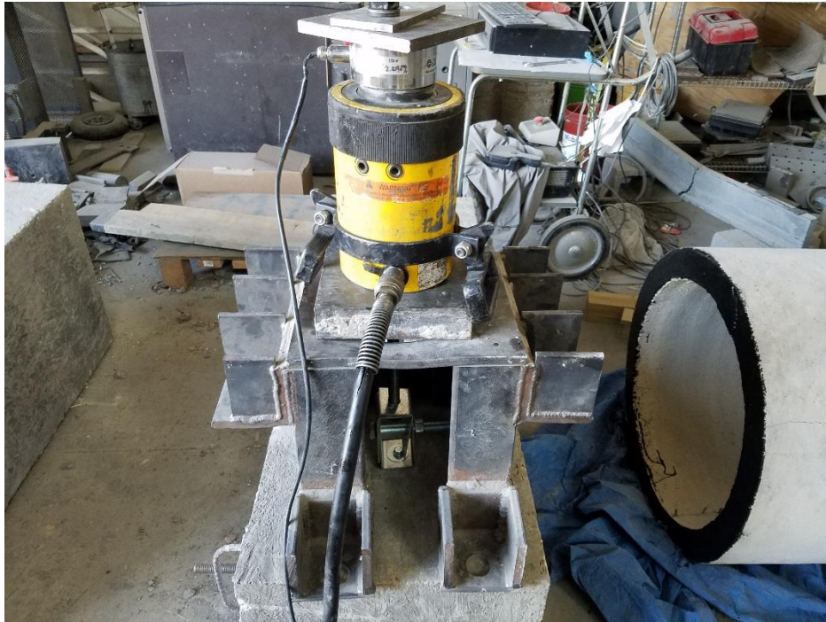
Figure 17: Anchor pullout test setup
