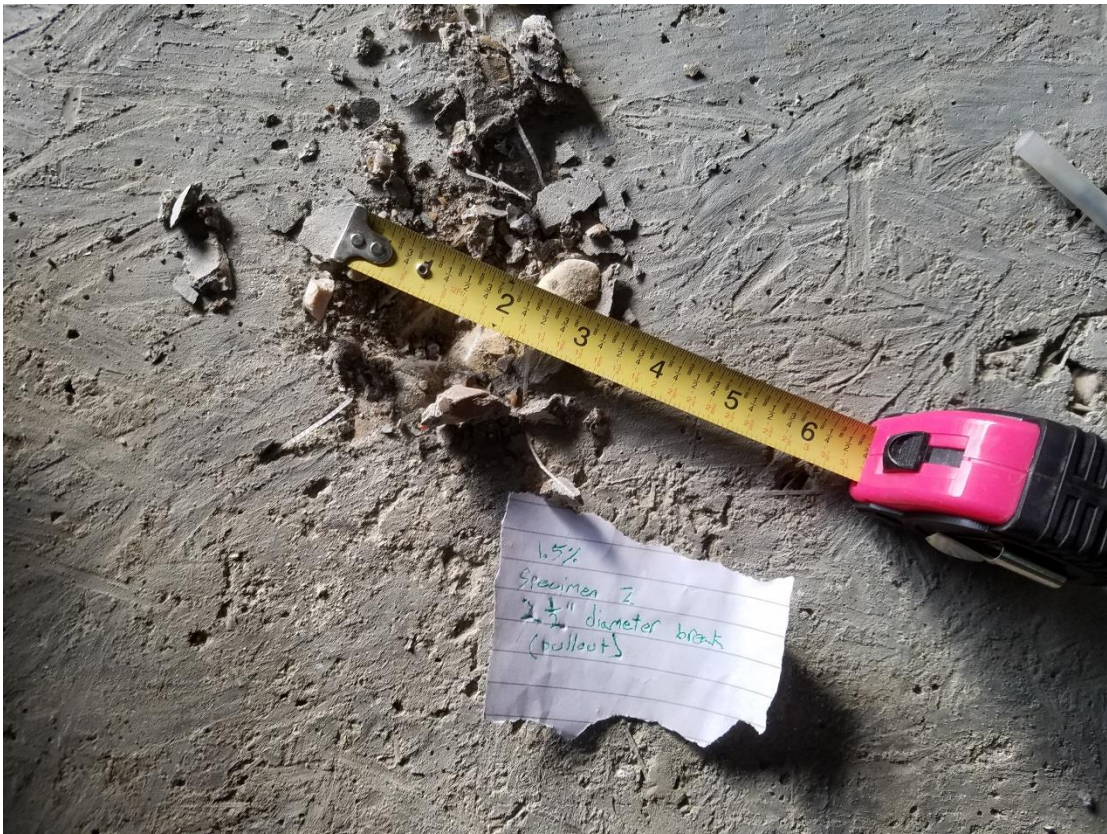
Figure 48: 1.5% Fiber - Specimen 2 Failure
