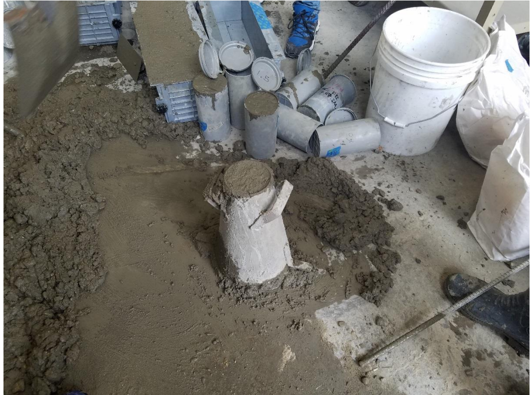
Figure 6: Filled Slump Cone
