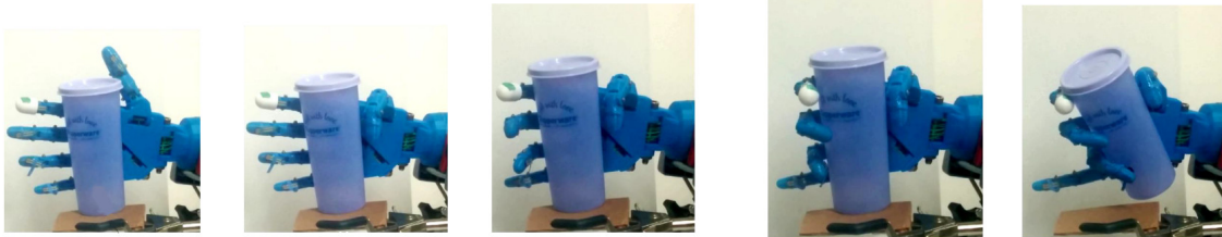
Figure 2.8: Time lapse images of the artificial hand grasping the unknown object based on input characteristics, [1].
