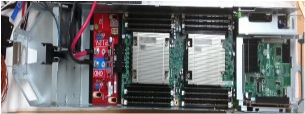
Figure 5 Top view of Open Compute Server
