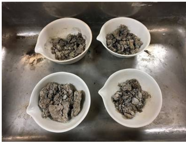
Figure 3-8 Residue or ash content of MSW after the ignition
