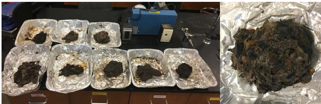
Figure 3-13 Degraded waste after dismantling
