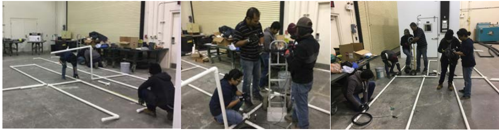
Figure 5-16 Sensor attachment with PVC pipe
