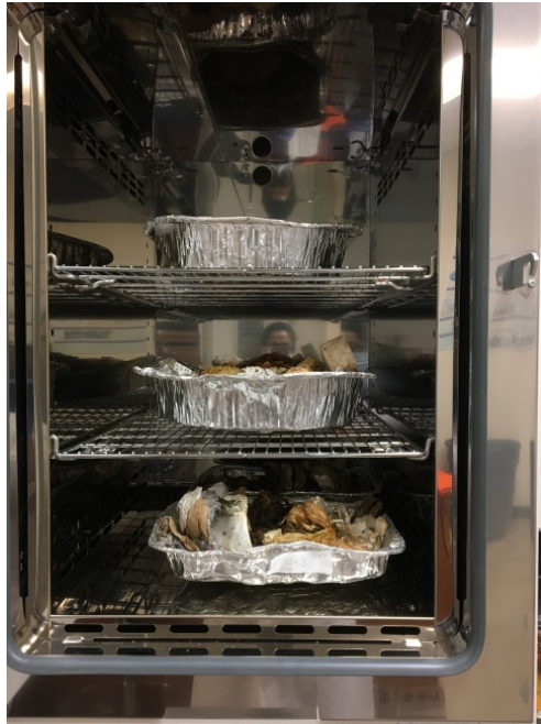
Figure 3-7 Determination of moisture content by drying sample in the oven
