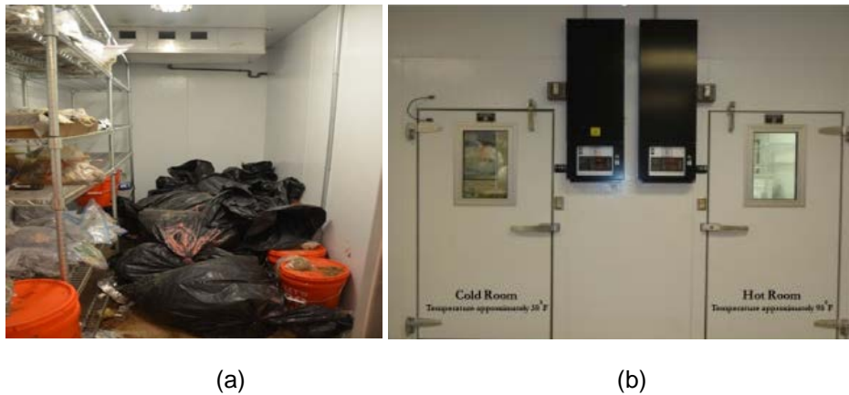
Figure 3-3 a) Stored sample in cold room; b) Environmental Growth Chamber (Cold room and hot room)
