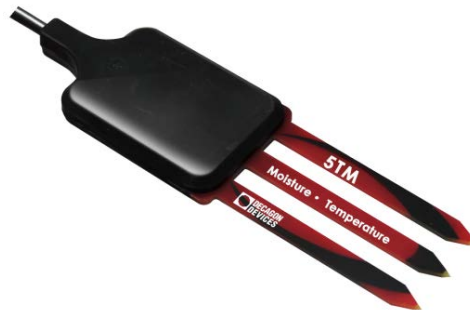
Figure 5-38 Moisture and temperature sensor 5TM (Decagon)
