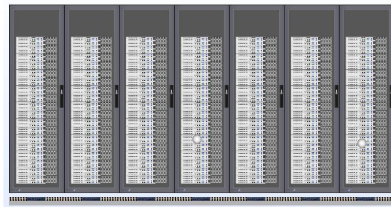
Figure 4-9 Sensor location on left side of the hot-aisle
