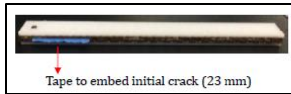
Figure 1-4 Modified DCB specimen for Peel Test [28]
