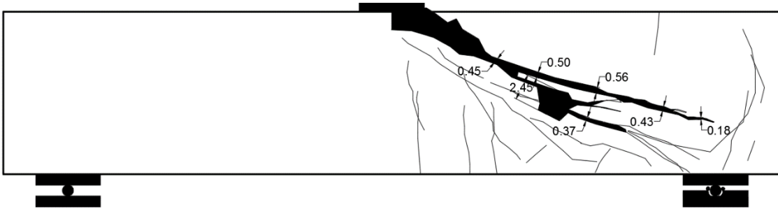
Figure 197 Crack pattern at failure for SNFRC 0.75% beam #31
