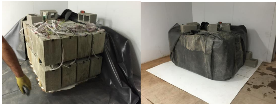
Figure 35 Typical photo of eight large-scale beams wrapped with PVC pan liner
