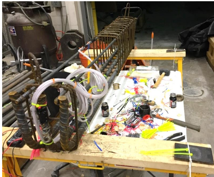
Figure 17 Typical photo of steel strain gage installation
