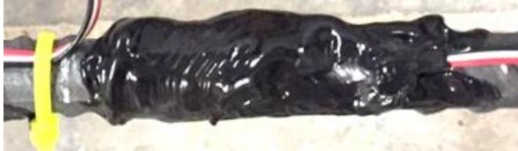
Figure 16 Typical photo of steel strain gage protected with a liquid electric tape
