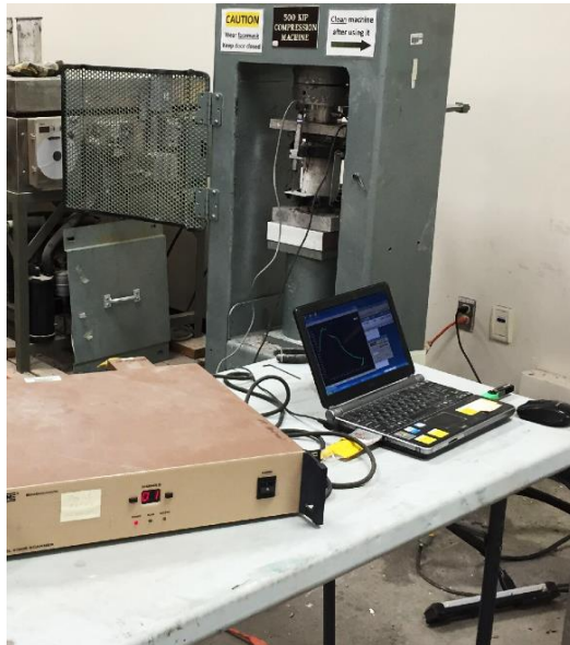
Figure 44 Typical photo of data acquisition for compressive cylinders
