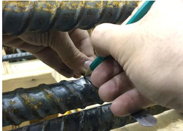
Figure 11 Typical photo of alignment of steel strain gage preparation with a 4H pencil
