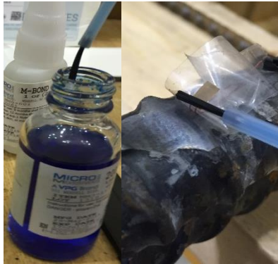
Figure 12 Typical photo of strain gage installation with M-Bond 200 catalyst
