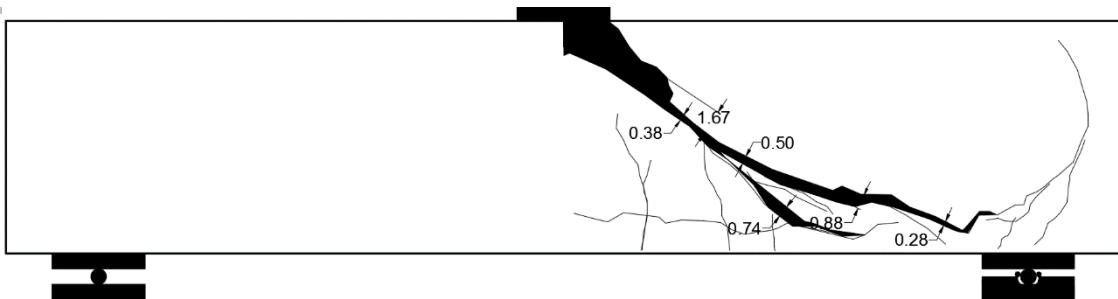
Figure 198 Crack pattern at failure for SNFRC 0.75% beam #32
