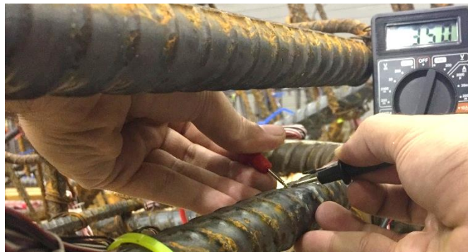
Figure 13 Typical photo of testing the resistance of steel strain gages
