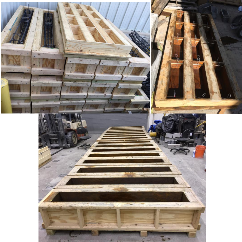
Figure 6 Typical photo of formworks used in this study
