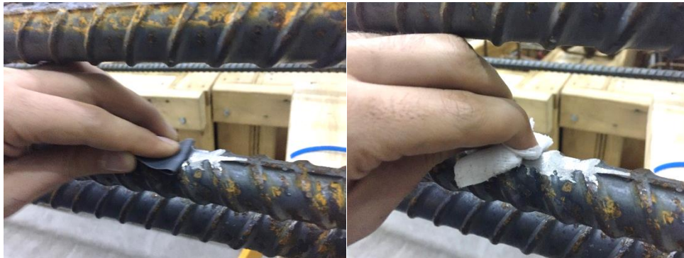
Figure 10 Typical photo of surface preparation of steel strain gages
