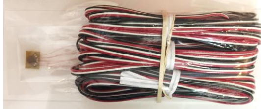
Figure 22 Typical photo of general purpose stacked rosette strain gage used on the surface of concrete beams in this study
