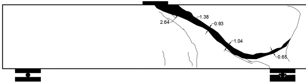
Figure 180 Crack pattern at failure for SNFRC 0.5% beam #14
