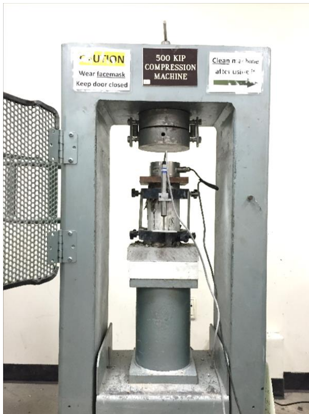
Figure 43 Typical photo of a 500 kip compression machine for compressive cylinders
