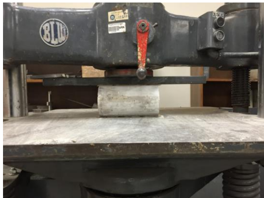
Figure 45 Typical photo of splitting test for cylinders
