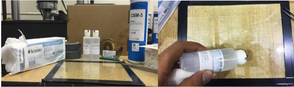
Figure 9 Typical photo of surface preparation for placement of steel strain gages
