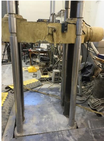
Figure 38 Typical photo of Universal Testing Machine with a capacity of 400 kips
