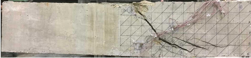
Figure 477 RC control BM# 17
