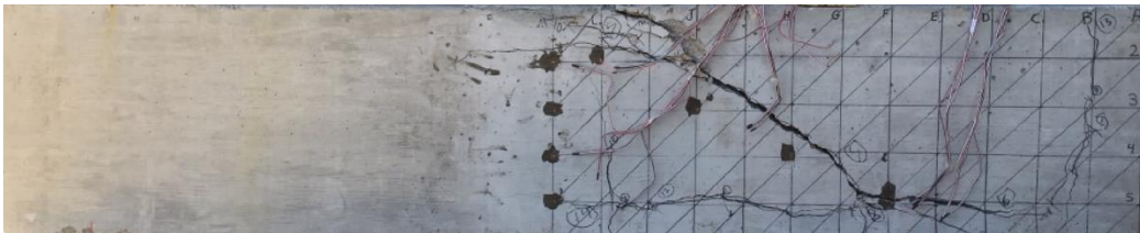
Figure 54 Typical photo of RC control beam at failure
