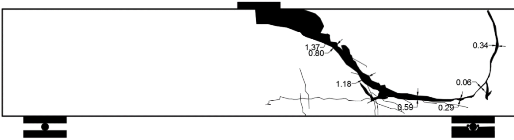
Figure 175 Crack pattern at failure for RC beam #9
