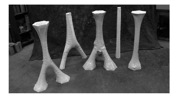
Figure 6-10 Final cast columnar specimens
