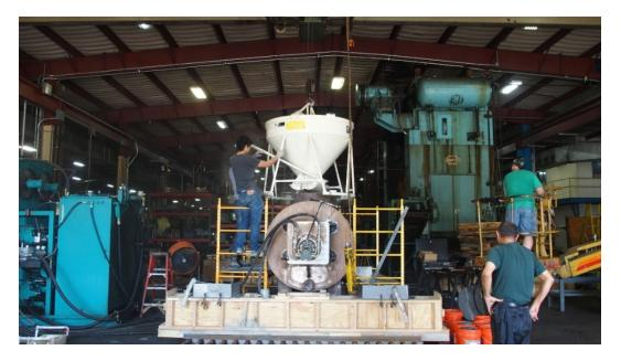
Figure 3-16 Special hydraulic concrete mixer used for casting of beam UHP-FRC #1
