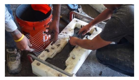
Figure 3-18 Direct tensile test specimens for UHP-FRC
