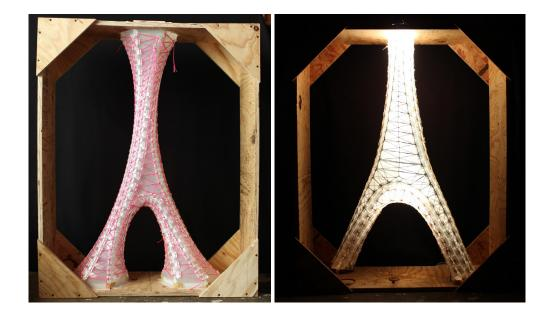
Figure 6-7 Semi rigid form with wooden scaffolding
