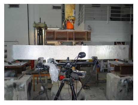
Figure 3-24 A view of test setup and CCD cameras mounted for DIC
