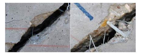
Figure 3-2 Lumpy distribution of fibers due to undissolved adhesion (Cho, 2011)
