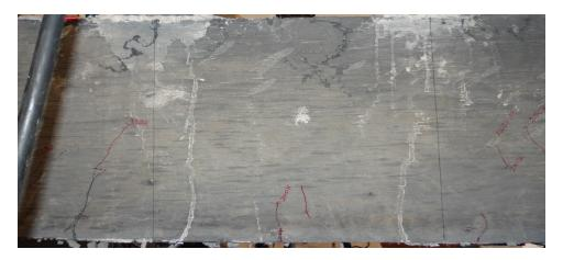
Figure 4-1 Compression zone damage of beam UHP-FRC #1 at 318 kips (peak load)
