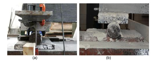
Figure 3-22 (a) Roller support (b) Hinge support
