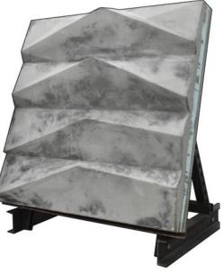
Figure 7-3: UHP-FRC Waffle Panel (Panel 3)
