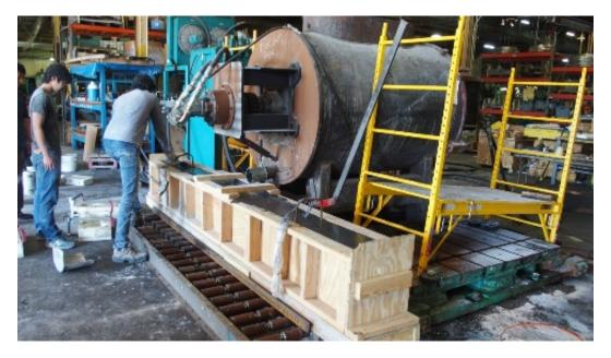
Figure 3-17 Cast beam UHP-FRC #1
