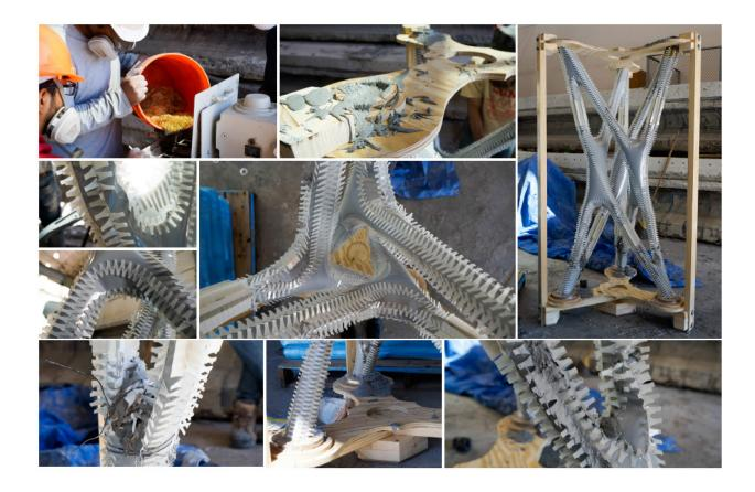
Figure 6-25 Final casting of 38" x 33" x 68" columnar branch
