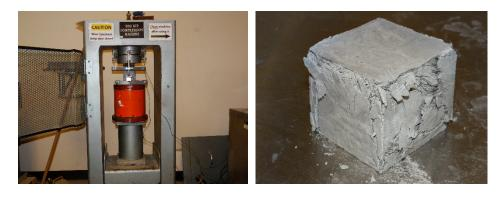
Figure 3-32 (a) Compression test machine and setup (b) Typical crushing of cube at the end of testing (7% strain)
