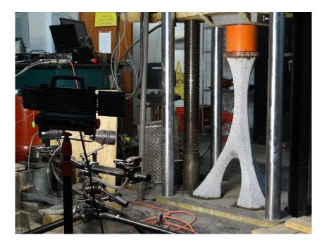
Figure 6-14 Test setup for RC columnar structure
