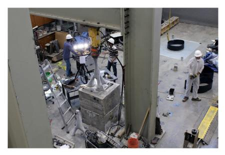
Figure 6-13 Experimental test setup with UHP-FRC column #2 in place
