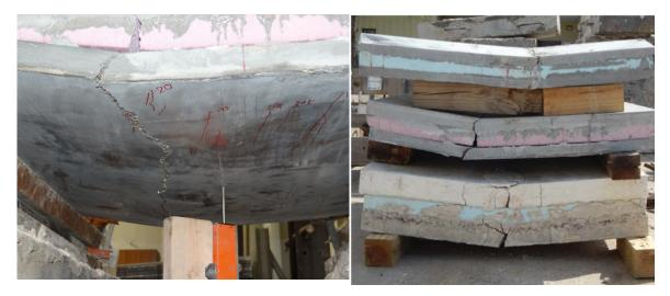
Figure 7-16: Cracking at peak load
