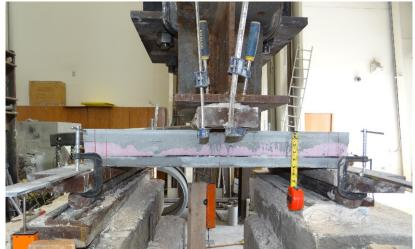
Figure 7-13: 3 point bending test
