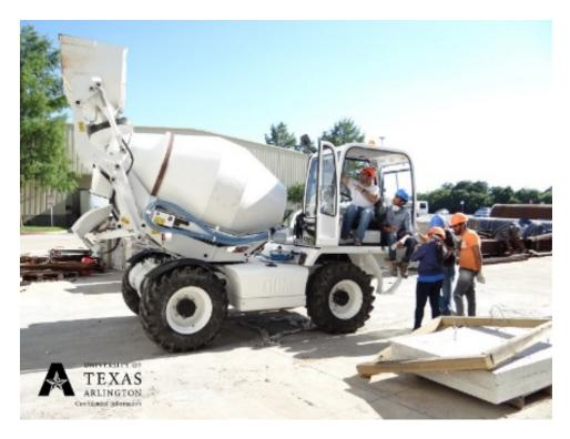
Figure 3-19 Concrete mixer truck used for casting beams UHP-FRC #2, #3, #4 and #5
