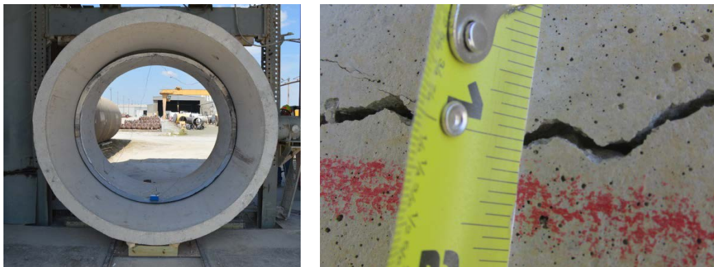
Figure 5-51 - Collapse of the CFRP internal coupler for TW-84-0.375 specimen
