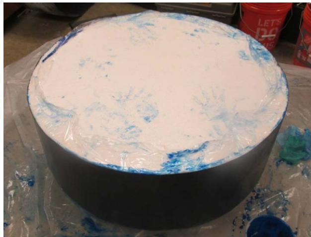
Figure 5-24 - 36-inch Styrofoam wrapped by the CFRP fabric sheet
