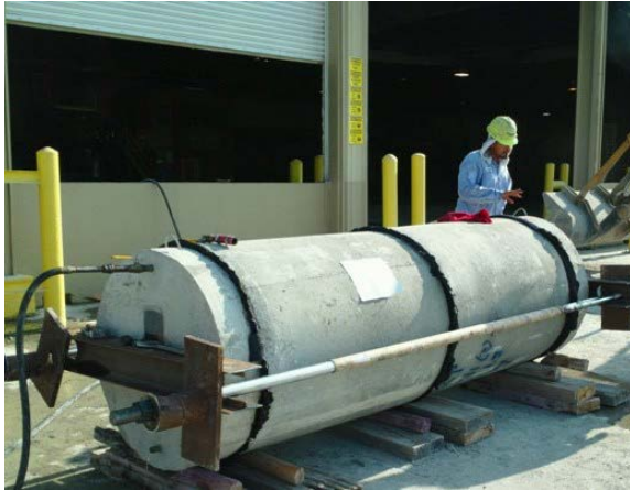
(a) Hydrostatic testing
