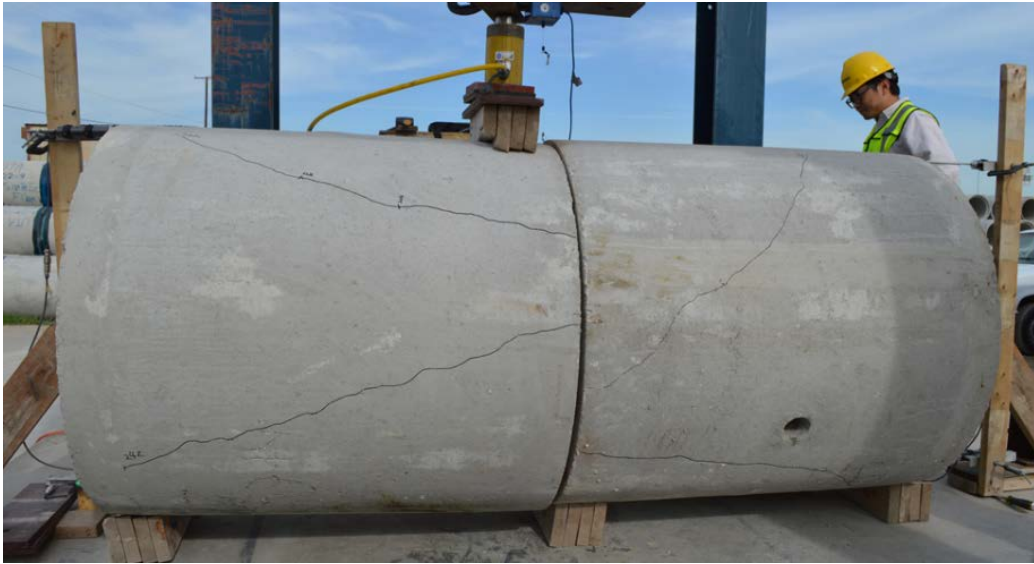
Figure 5-30 - Propagated crack pattern on springline of pipes at 24 kips for 36-inch RCP
