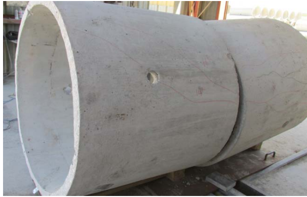
(a) Full-scale experimental joint shear test on 48-inch pipe
