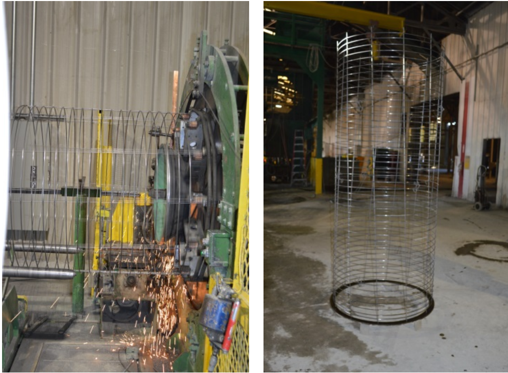
Figure 5-2 - Production of steel cages: (a) Welding machine (b) Steel cage
