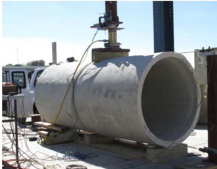
Figure 5-25 - Experimental joint shear test setup for CFRP internal coupler
