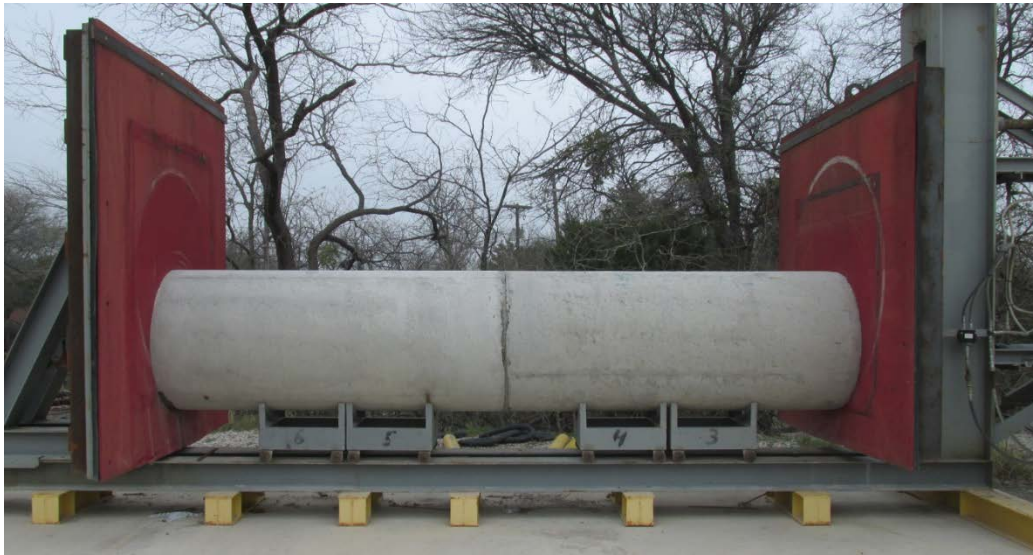
Figure 5-57 - Hydrostatic test setup
