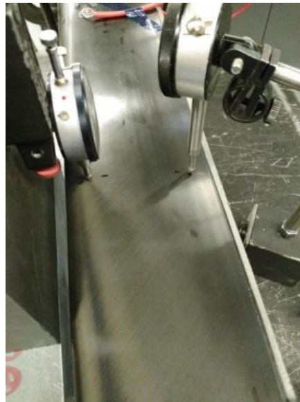
Figure 5.12 Placement of dial gages for specimen 2
