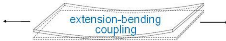
Figure 2.11 Laminate experiencing bending induced by normal load
