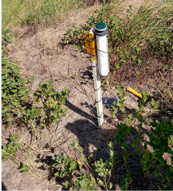
Figure 4.36: ETgage™ installed between Lysimeters 4 and 5 (inclined sections).
