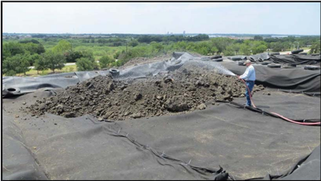
Figure A.161: Water placement on the soil pile in the middle top section lysimeter.
