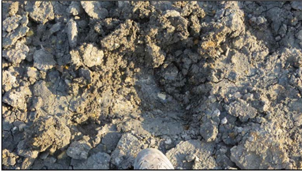
Figure A.169: Damp soil from excavating into the south top section (morning).
