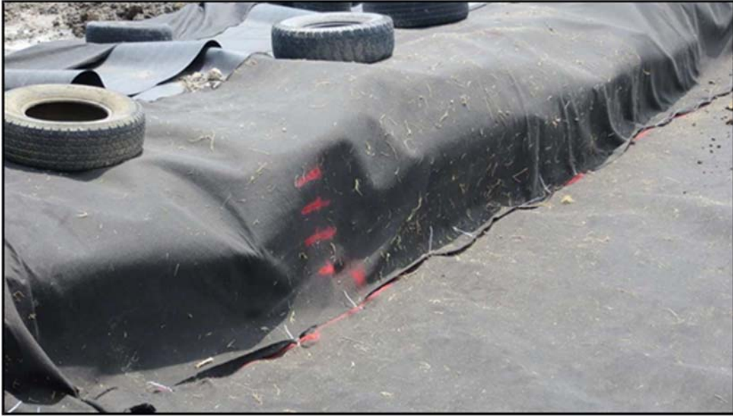
Figure A.162: Lift thicknesses marking in the middle top section lysimeter.
