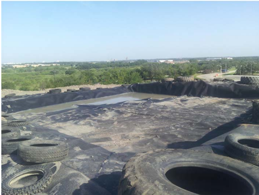
Figure A.116: North Top Section lysimeter on Monday (after Friday morning rainfall).
