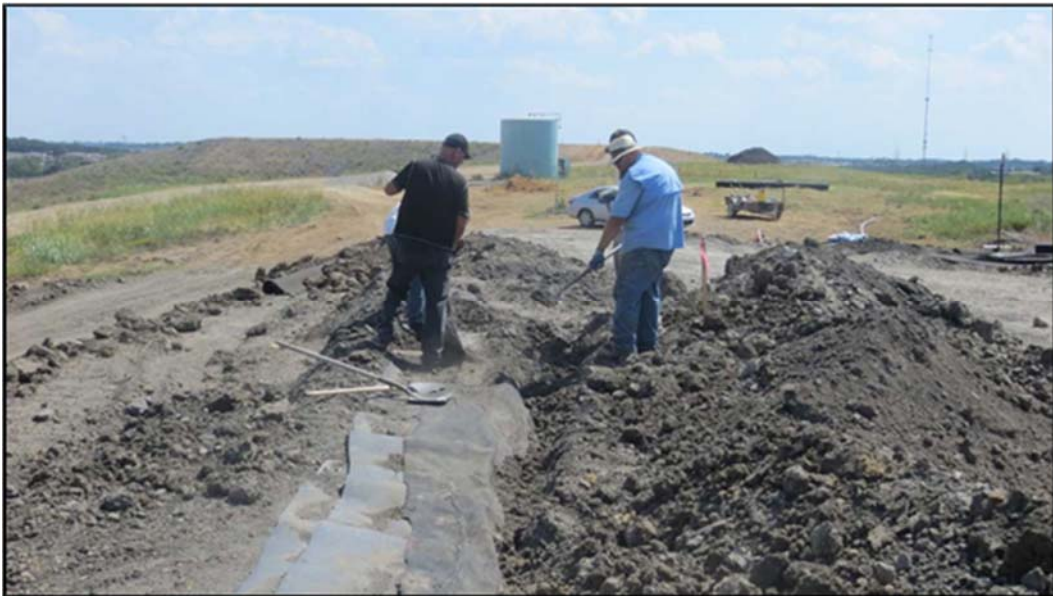
Figure A.329: Removing soil from the lysimeter boundaries-two (2).
