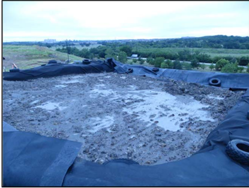
Figure A.204: Soil pile details in the middle top section lysimeter after a rainfall event.
