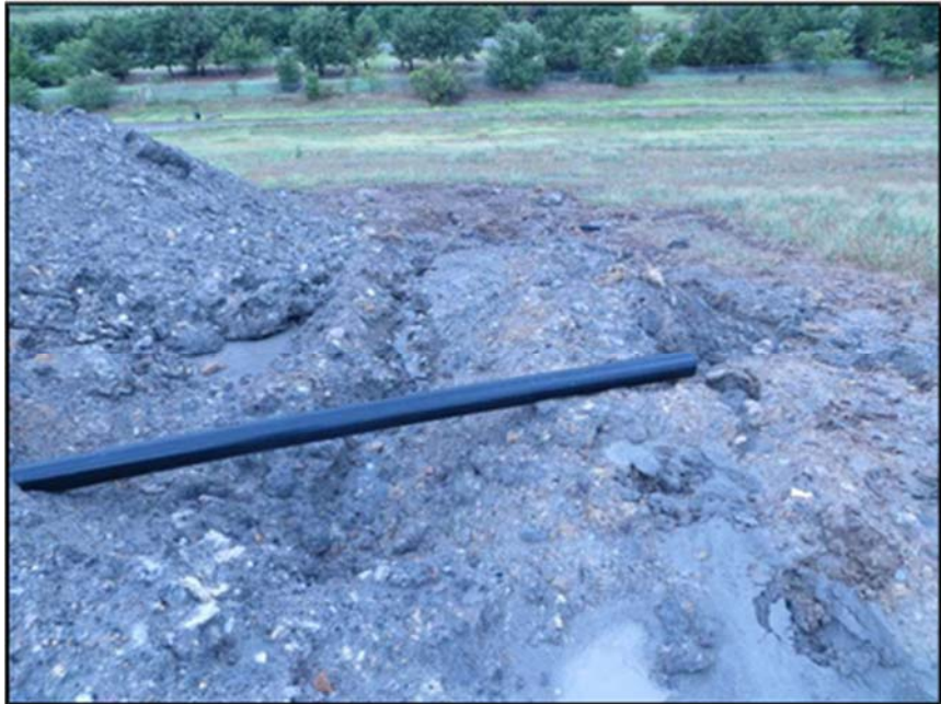
Figure A.183: Gullies formed by the flow of water from the middle and north top sections.
