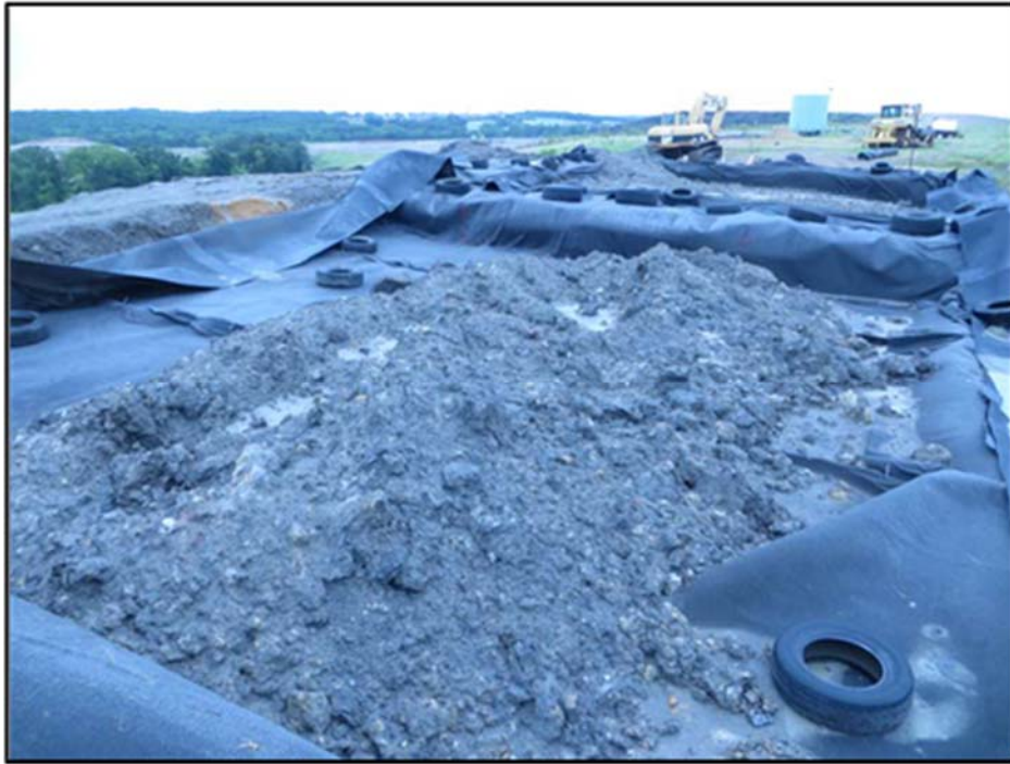
Figure A.203: Soil pile details in the north top section lysimeter after a rainfall event.
