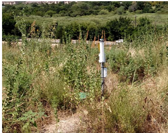
Figure 4.37: ETgage™ installed between Lysimeters 1 and 2 (top sections).
