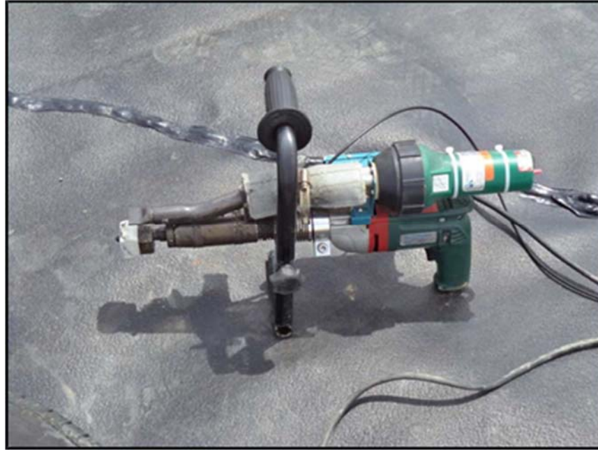
Figure A.101: Replacement extrusion welder (MINI-Z – Extrusion Welder from Polyweld USA).
