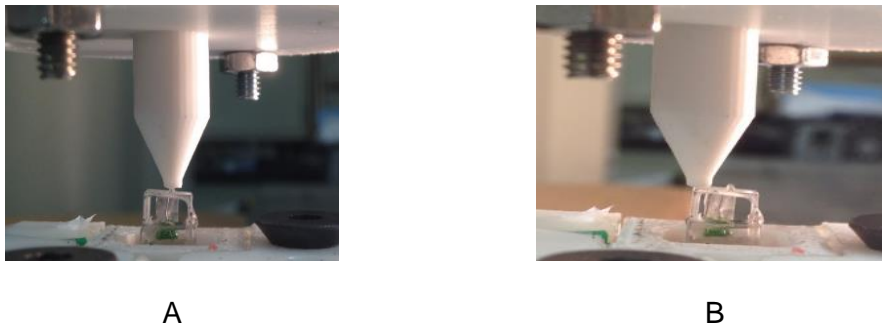
Figure 65: Applied displacement ( 40\ \mu m ) at the vertical force sensing structure for experimental verification. A, Center of the vertical force sensing structure. B, End of the vertical force sensing structure
