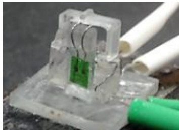
Figure 46: Assembly of vertical and horizontal force sensing structures
