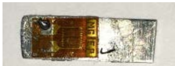
Figure 32: Strain gauge attached on the scaled aluminum prototype beam model
