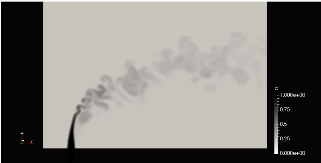
Figure 6.3. Figure showing the instantaneous center plane scalar concentration.
