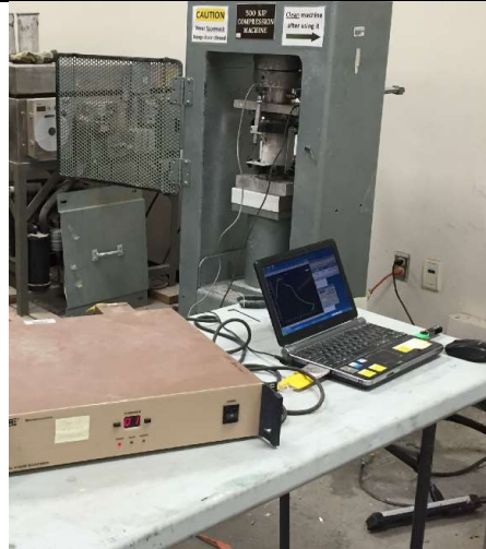
Figure 41 Compression test data acquisition network
