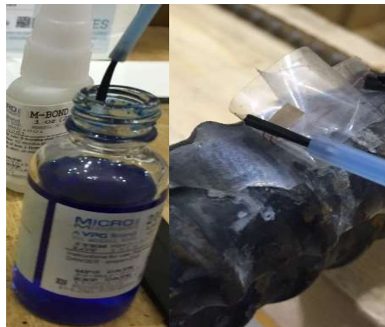
Figure 13: Catalyst applied to bonding side of strain gage
