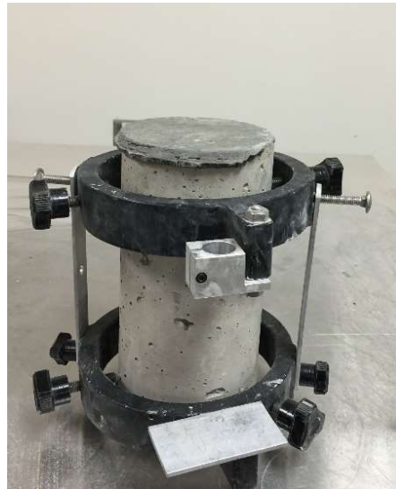
Figure 39 Testing jig mounted to cylinder for compression test
