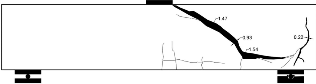
Figure D5 Crack pattern at failure for SNFRC 0.5% beam #5
