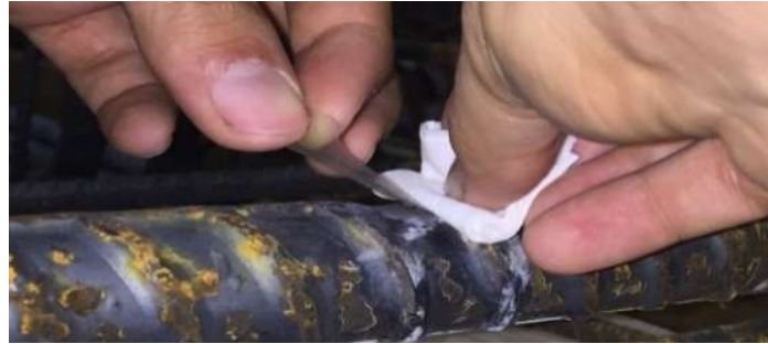
Figure 14 Removing the tape from the gauge assembly
