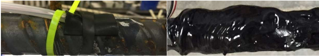
Figure 18: waterproof and UV-resistant sealed strain gage assembly
