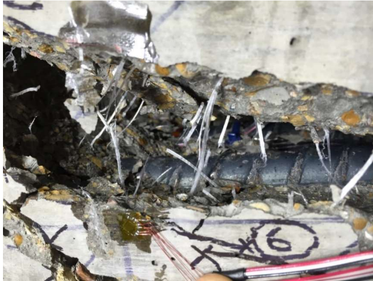
Figure 45 Pullout resistance and rupture of fibers in SNFRC beams
