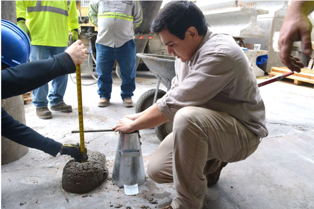
Figure 28 Slump test performed on-site
