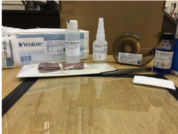
Figure 12 Steel strain gage installation kit
