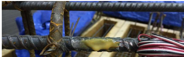
Figure 17 M-Coat B coated strain gauge
