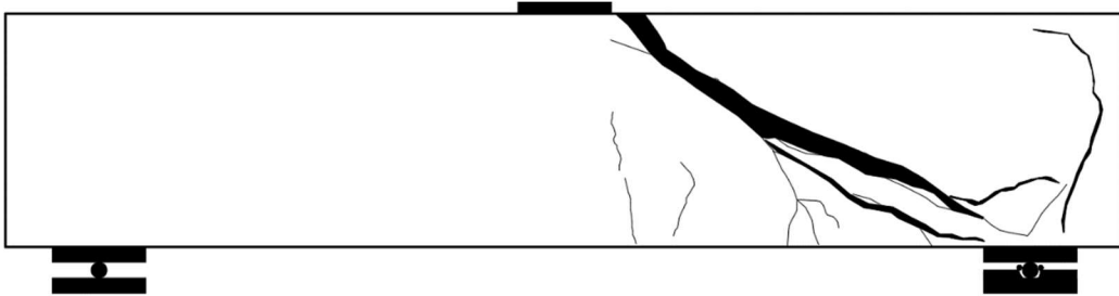
Figure D7 Crack pattern at failure for SNFRC 0.75% beam #7
