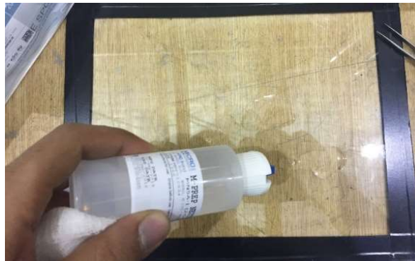
Figure 10 Neutralizing a smooth glass surface
