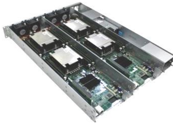
Figure 30: 3 rd generation Open Compute server [20]
