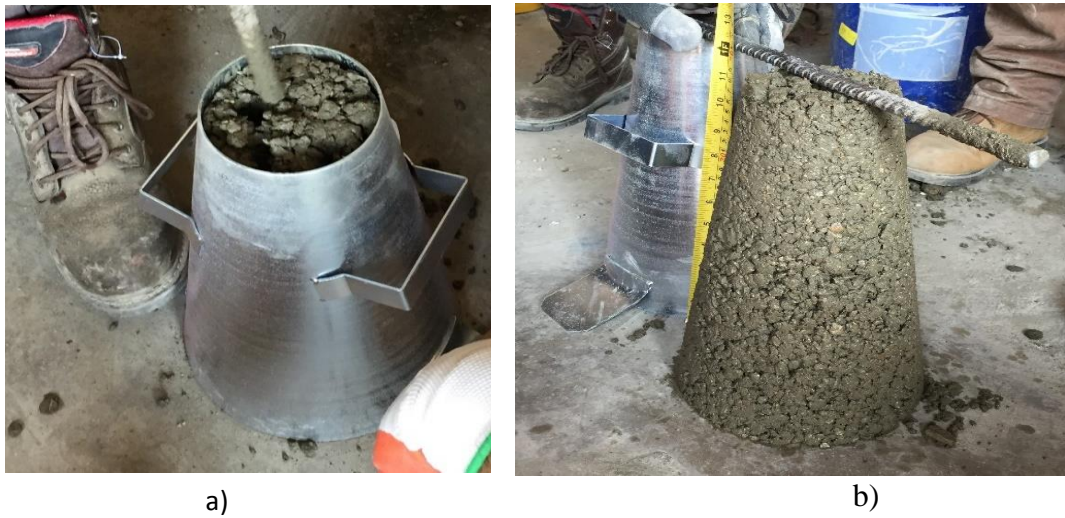
Figure 2.5 - (a) slump test (b) zero-slump dry cast concrete
