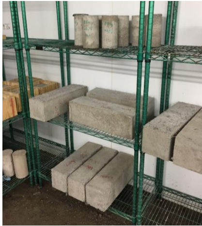
Figure 2.7 - Placing specimens in curing room for a duration of 7 days
