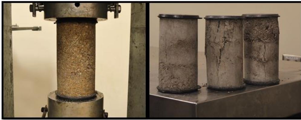
Figure 2.15 - Concrete compression test based on ASTM C39
