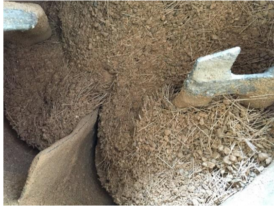
Figure 2.2 - Introducing synthetic fibers into the mixer after all dry aggregates
