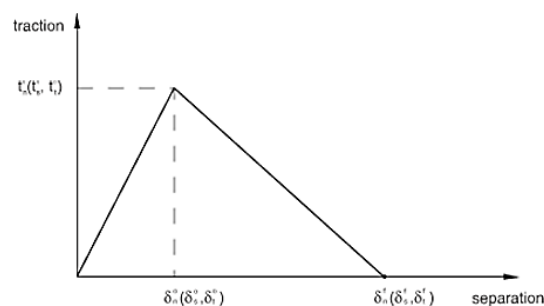
Figure 4.8 - Typical traction-separation behavior in cohesive elements [30]
