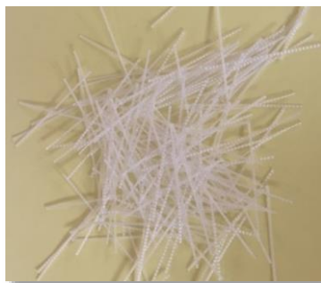
Figure 2.1- MasterFiber MAC Matrix synthetic fibers
