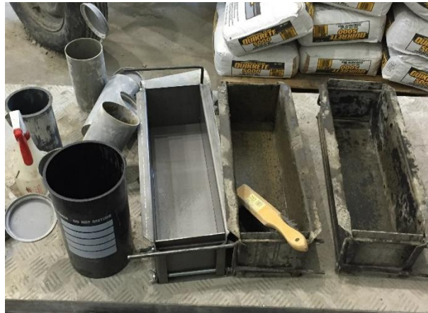
Figure 2.4 - A light coat of mold release used inside the molds
