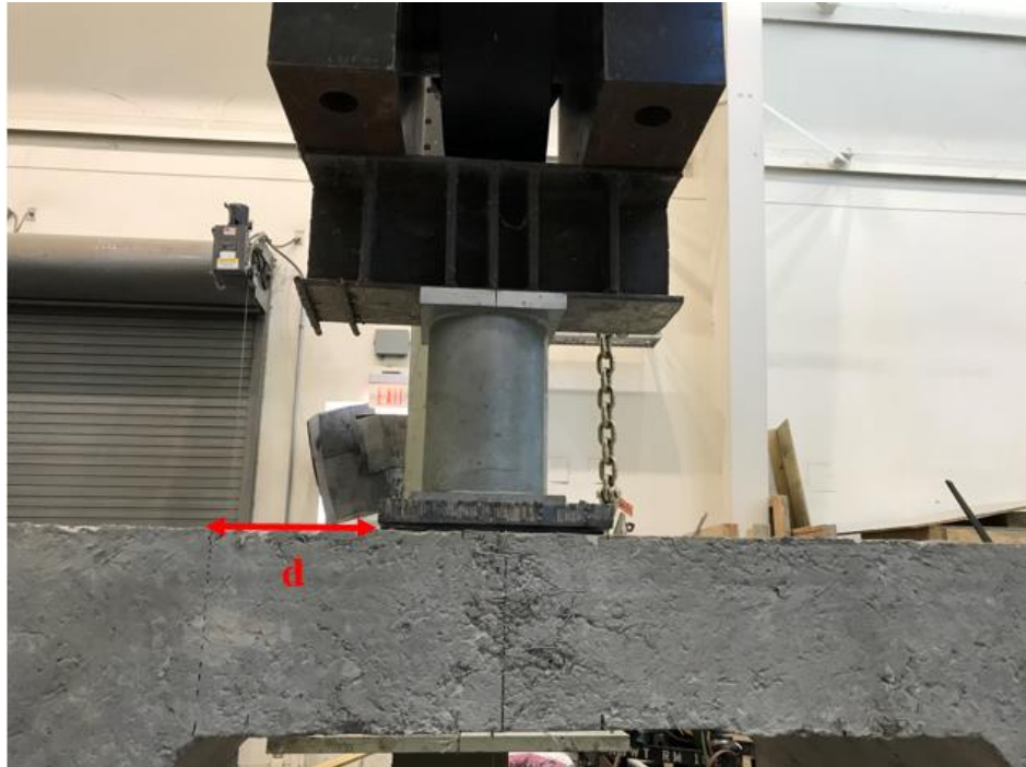
Figure 3.7 -The steel plate placed at the distance d in order to investigate the shear capacity of box
