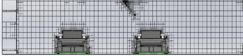
Figure 3-2 Adaptive mesh refinement cut plot
