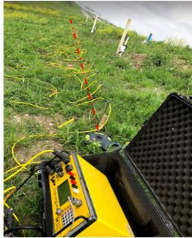
Figure 5-31. 2D Resistivity imaging line.
