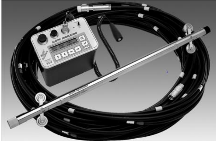
Figure 4-6. Slope indicator (vertical inclinometer).
