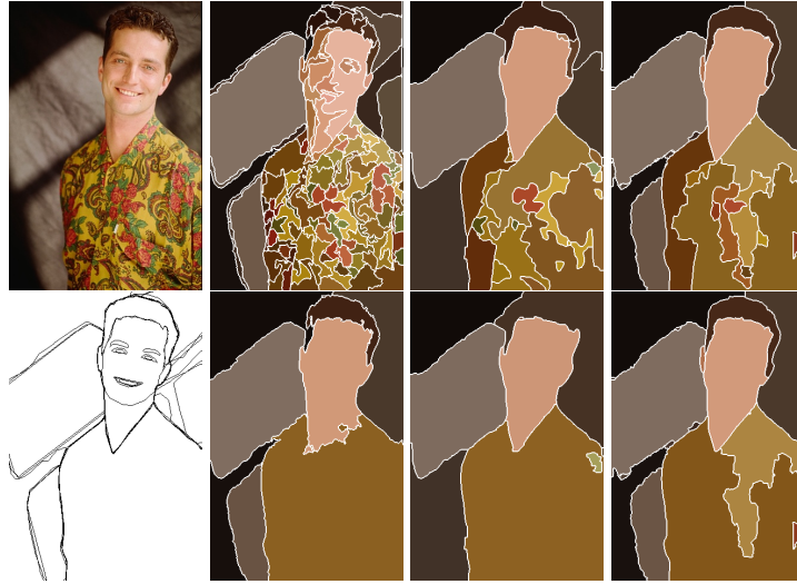
Figure 2.4: IS4 in combination with different over-segmentation. From left to right, top row: image, CCP-2 [1], ISCRA [2], and MCG [3]; bottom row: groundtruth, IS4(CCP-2), IS4(ISCRA), and IS4(MCG); The top row shows the initial over-segmentation provided by these methods and the bottom column shows our final segmentation with these initial over-segmentations.
