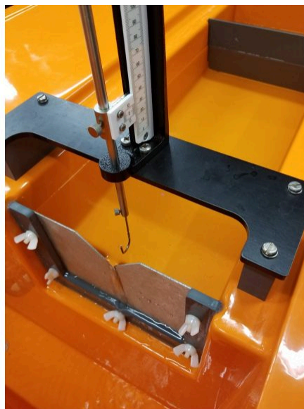
Figure 9.3: Position of the notch and Vernier height gauge to set the datum.
