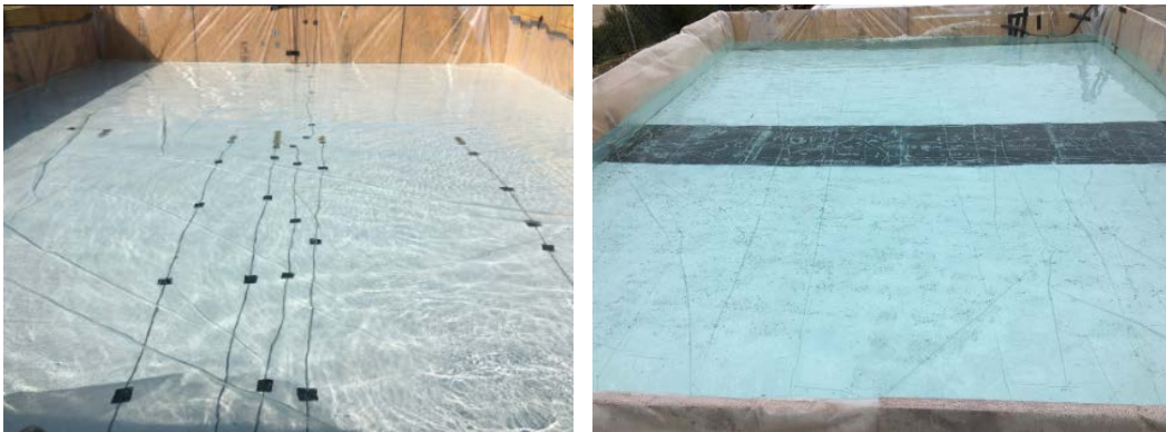
Figure 4-18 Load test on the control (left) and the strengthened specimen (right)
