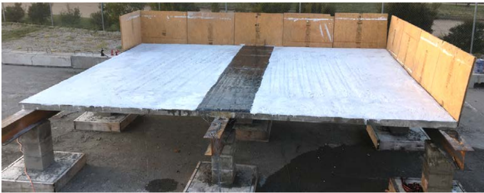
(a) CFRP-strengthened slab after load test
