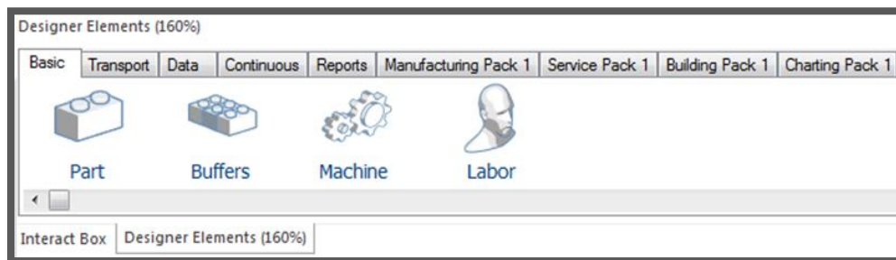
Figure 4-11 Main Elements: Part, Buffers, Machine, and Labor. Created with WITNESS™ (Lanner Group, 2008) software
