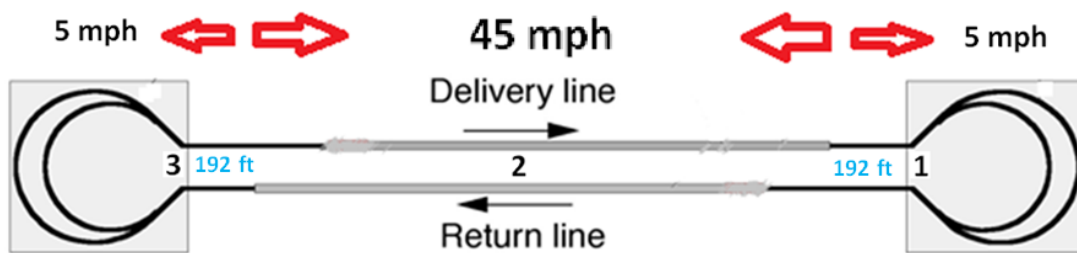
Figure 4-7 Speed Changes into Three Parts and Braking Distance in the Terminal Entrance
