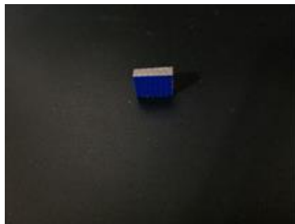
Figure 12-2 Cut section image of PCB for SEM
