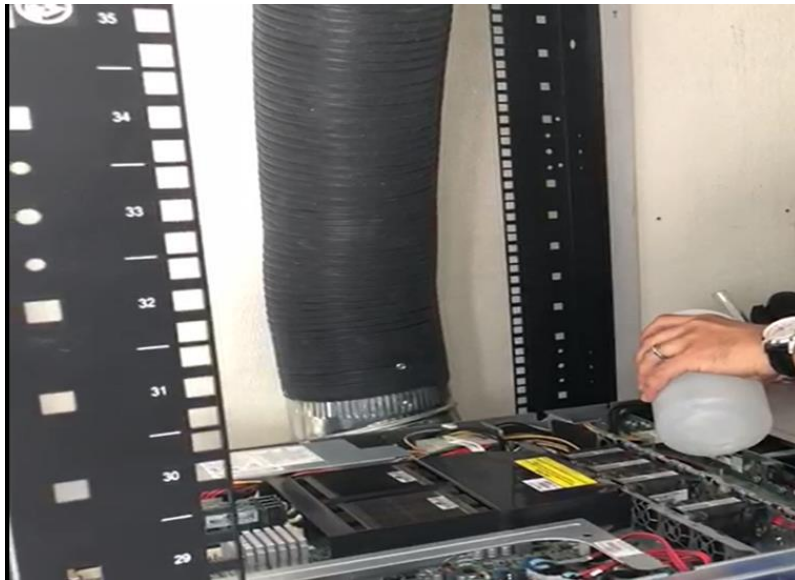
Figure 6-1 Collecting samples using Deionized water
