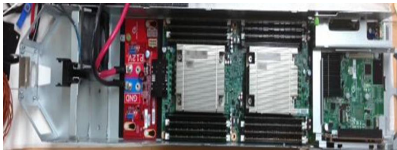
Figure 9-1 Top view of Open Compute Server
