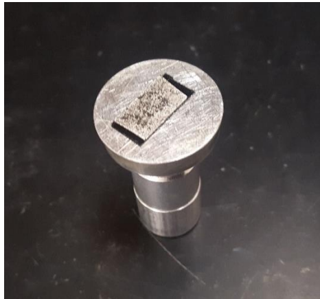
Figure 4-5: Sample holder with the silver-coated sample
