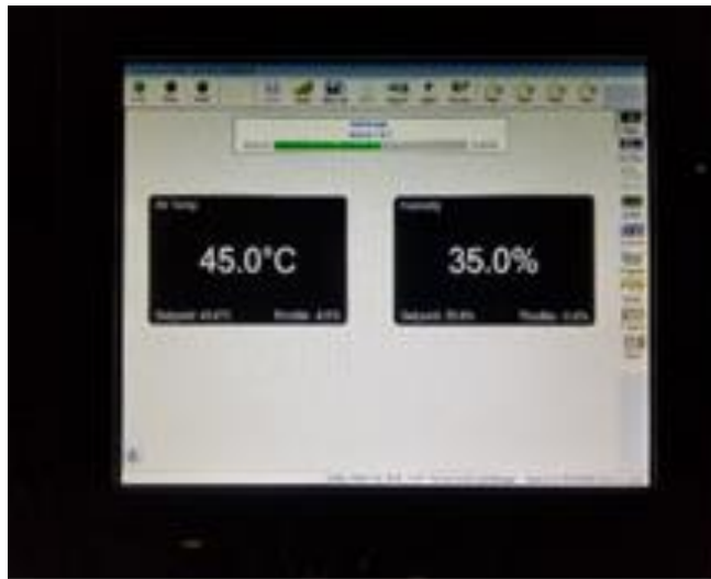
Figure 12-10 Thermotron display with environmental chamber conditions
