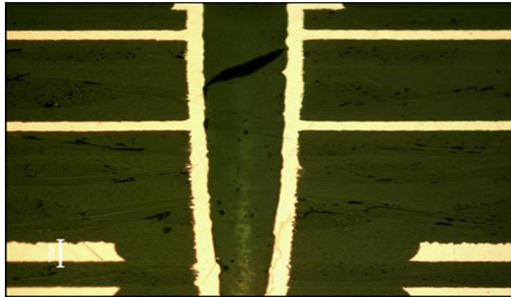
Figure 10-5 Cross section of PCB plated through-hole on oil exposed server
