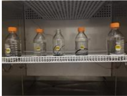
Figure 12-9 Environmental chamber containing the synthetic and mineral oil jars with components
