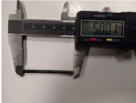
Figure 12-7 Air-Exposed Fiberoptic Cable Sample
