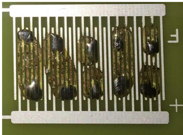
Figure 5-23 Corrosion due to the conducting nature of the NaCl salt solution at a relative humidity higher than the DRH.
