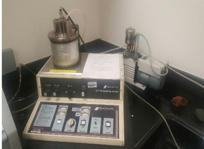
Figure 4-4: CrC 100 Sputtering System coating the non-conductive samples with silver
