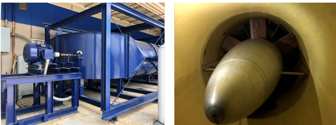
Figure 2.1: Low Speed Wind Tunnel of the Aerodynamics Research Center at the University of Texas at Arlington
