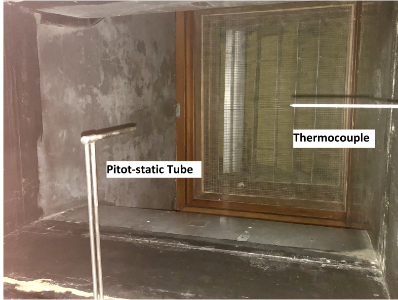
Figure 2.2: Pitot-static probe and K-type thermocouple in the test section
