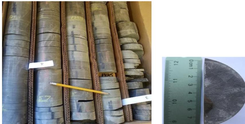
Figure 3-2 Prudential 1-A core in Marion County, Ohio: core box (left; photo from Ohio Geological Survey, Horace R. Collins Core Lab Facility located in Columbus, Ohio) and core plug (right) before they were cut.
