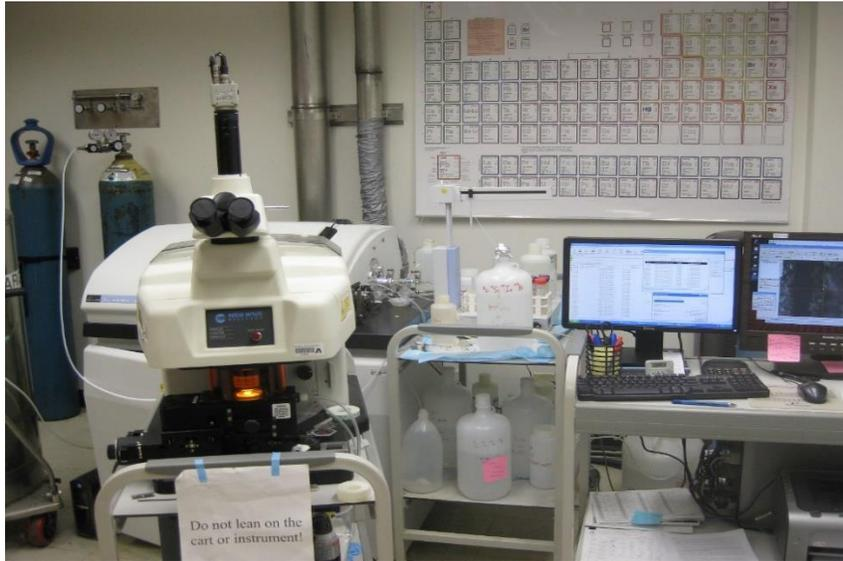
Figure 3-7 LA-ICP-MS apparatus for micro-scale elemental mapping
