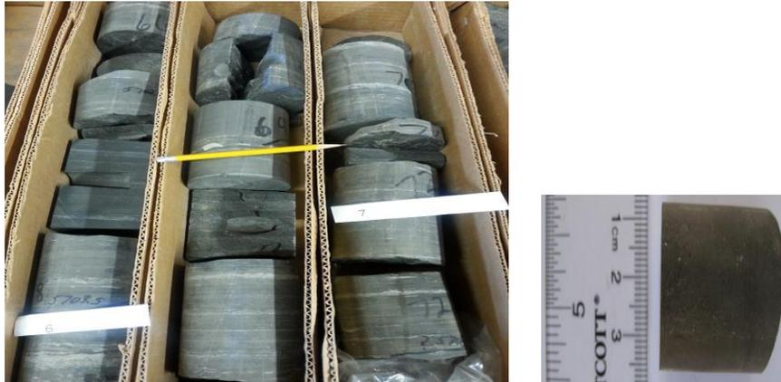
Figure 3-3 Fred Barth #3 core in Coshocton County, Ohio: core box (left; photo from Ohio Geological Survey, Horace R. Collins Core Lab Facility located in Columbus, Ohio) and core plug (right) before they were cut.
