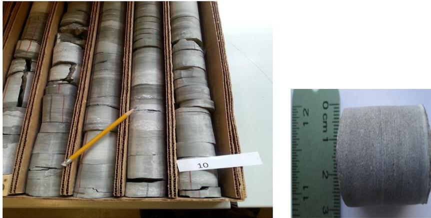
Figure 3-1 Goins # GS-3 core in Highland County, Ohio: core box (left; photo from Ohio Geological Survey, Horace R. Collins Core Lab Facility located in Columbus, Ohio) and core plug (right) before they were cut.
