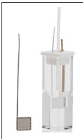
Figure 1-5 Schematic illustrations of the spectroelectrochemical cell and the platinum minigrid working electrode (Reprinted from reference 9).
