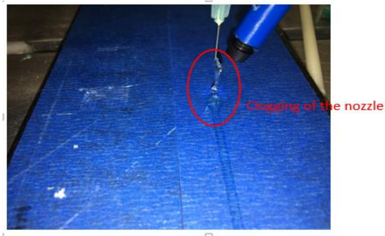
Figure 4.4 Clogging of the nozzle with LED mounted at angle of 35°
