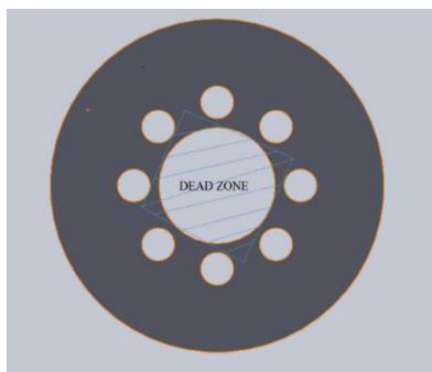
Figure 3.8 LED fixture plate with non-polymerizable area shown as Dead Zone
