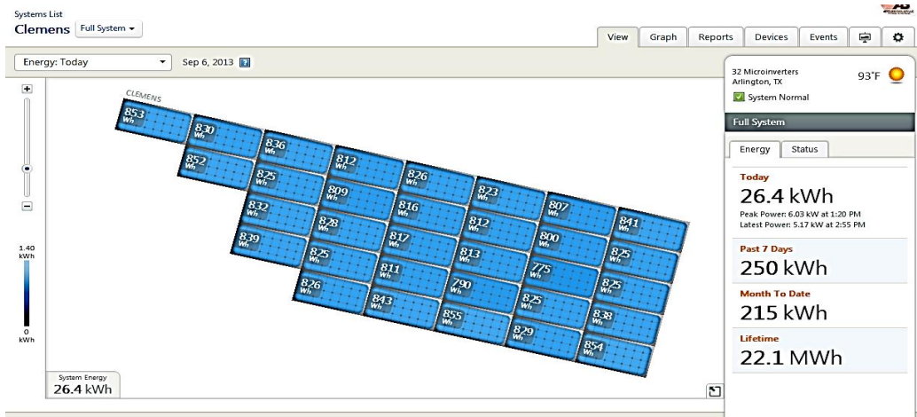
Figure 3.4 Base Solar System A; Data Monitoring
