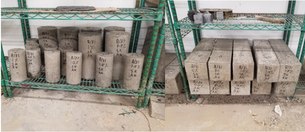
Figure 3- 10. Concrete Specimens Curing
