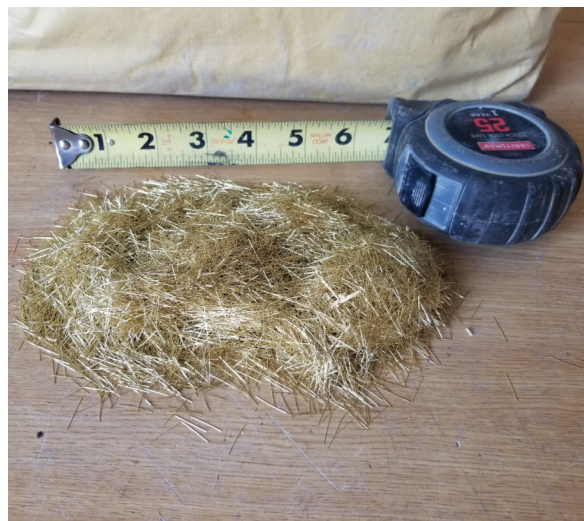
Figure 3- 1. (a). Steel Fiber DRAMIX bag (b) Steel Fibers DRAMIX 13/0.2
