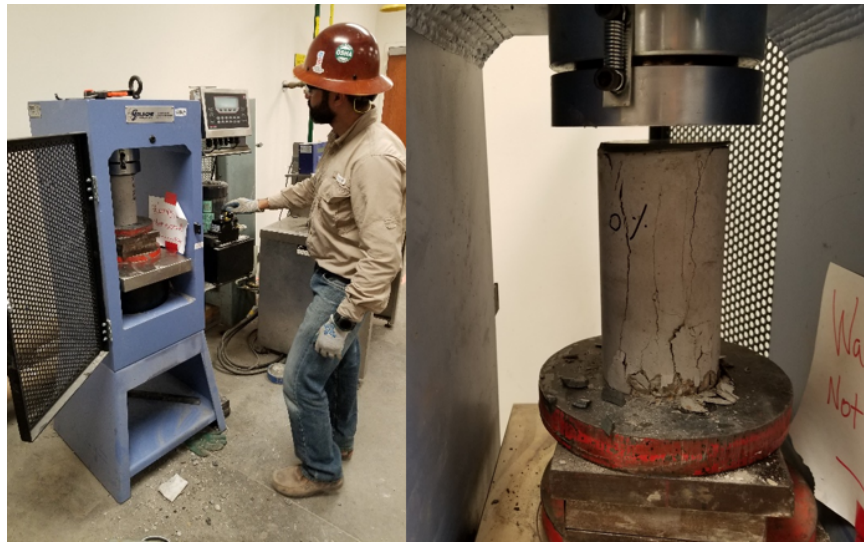
Figure 3- 11. compression test set up
