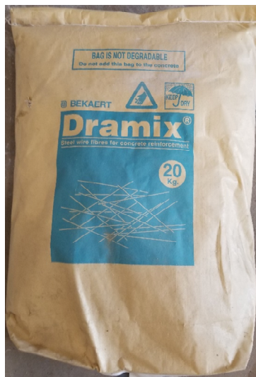
Figure 3- 1. (a). Steel Fiber DRAMIX bag (b) Steel Fibers DRAMIX 13/0.2
