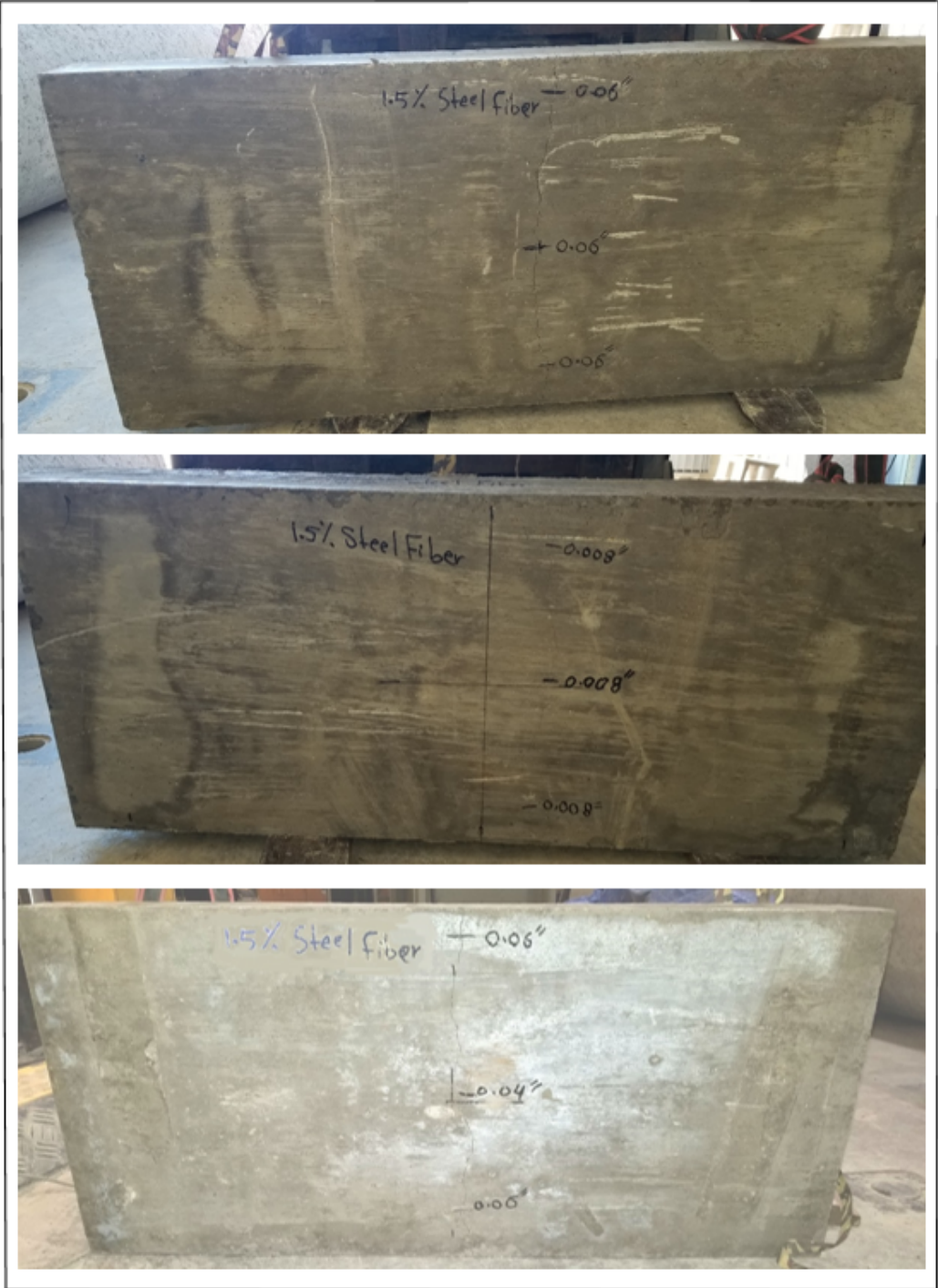
Figure 4- 16. Specimen Failure of SFRC (1.5%)
