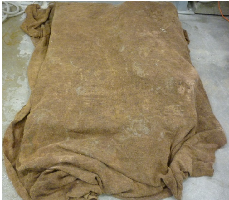
Figure 3- 9. Covering of the specimen after casting with wet cloth
