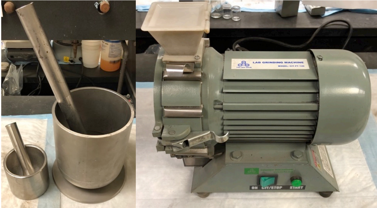
Figure 3-4: Mortar and pestle used to crush samples (left). Electric grinder used to crush samples (right).
