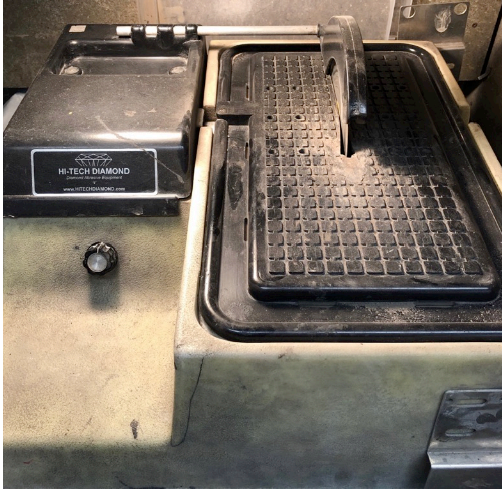
Figure 3-2: Hi-Tech Diamond saw used to cut samples.
