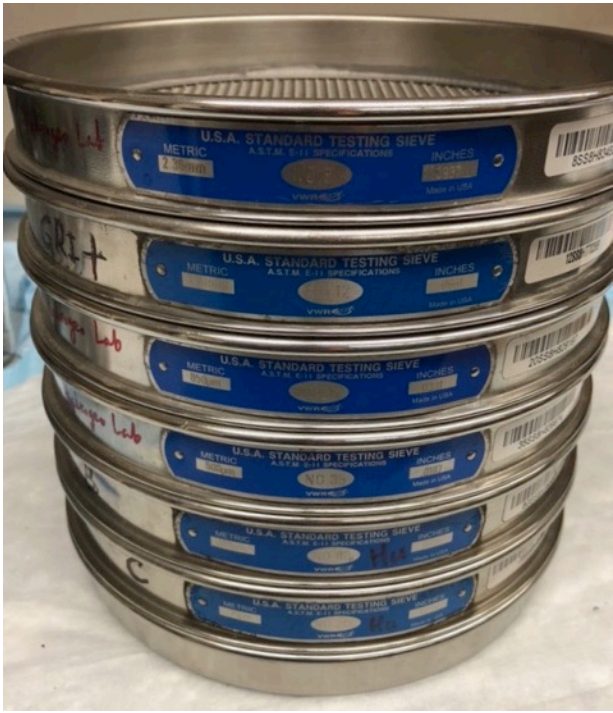
Figure 3-5: Sieve stack used to separate sample into discrete granular sizes.
