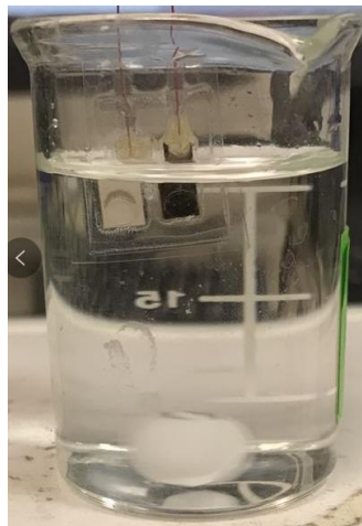
Fig 42 – Demonstration how laminated samples are tested in presence of magnetic stirrer.
