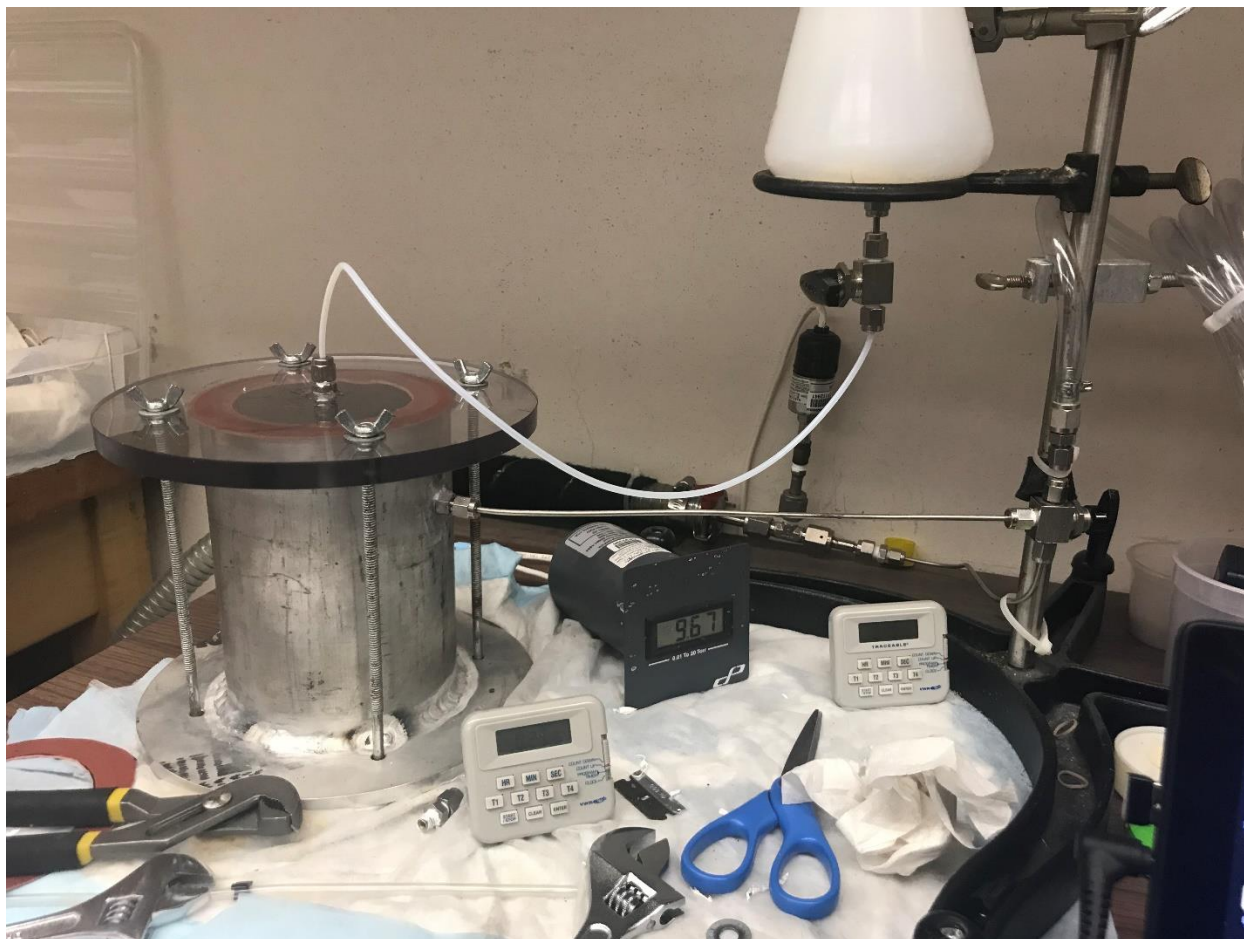
Figure 5: Vacuum Saturation Apparatus
