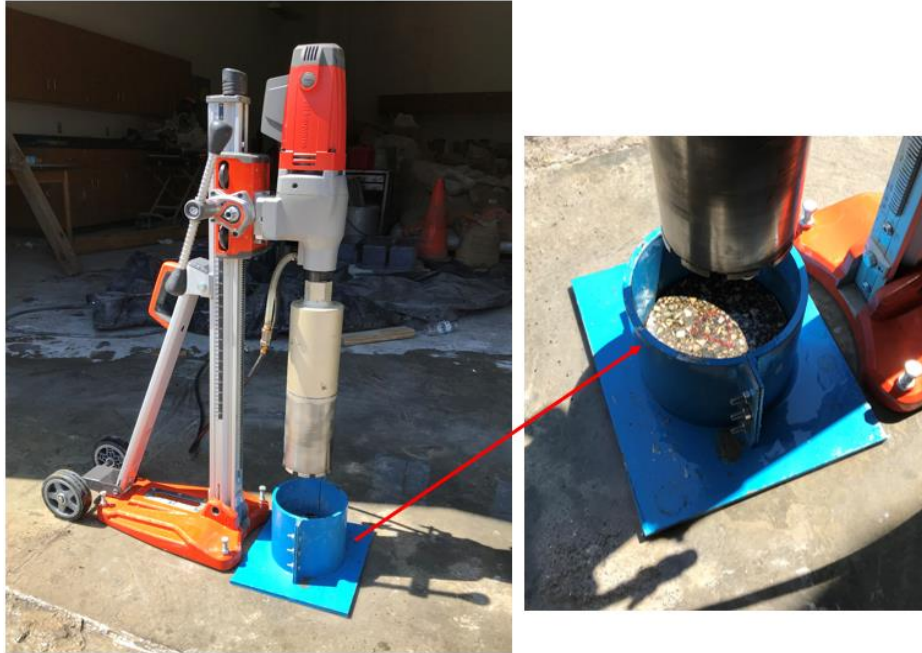
Figure 5-19. Coring Machine of the C4 Specimens.
