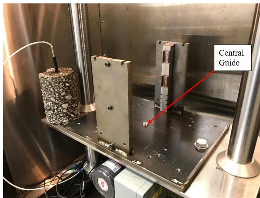
Figure 5-37. Installation of the DST Supporting Plate on the UTM-25 Loading table.
