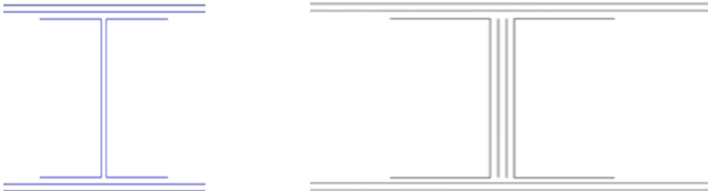
Figure7-2 and 4 bead 0° stiffened beam model cross section
