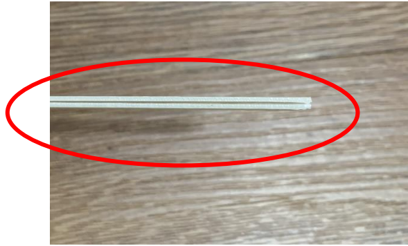
Figure 26-Gap between beads for tensile coupons
