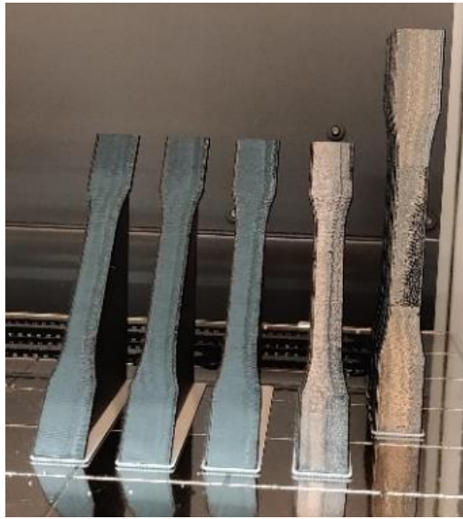
Figure 12-3D printed 90 0 and 45 0 test specimens and test configurations
