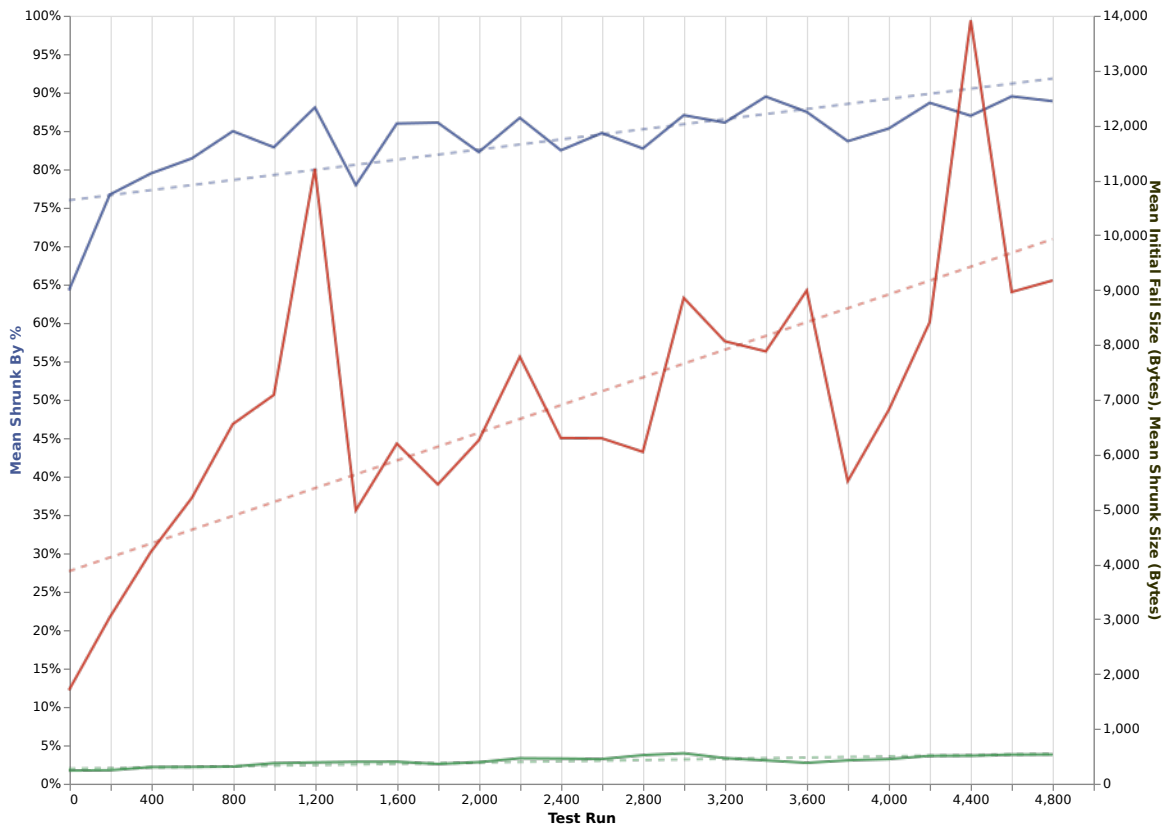
Figure 7.2: Plot of Firefox and Chrome testing runs (with reduction between runs) showing the mean initial failure size byte count (red), the mean final shrunken size byte count (green), and reduction percentage (blue). Linear regressions for each plot line are shown as dotted lines.
