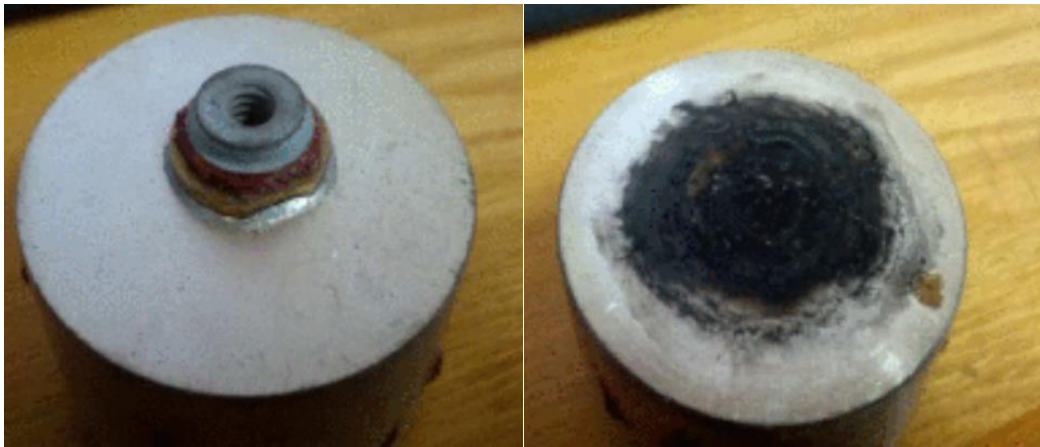
Figure 20: The brass terminals before and after lifetime tests [14]
