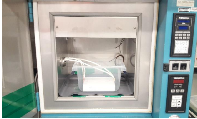
Figure 25: The Unit Under Test (UUT) capacitor will be placed inside a temperature chamber and will be submerged in oil. While in the temperature chamber, the UUT will be under various ambient conditions.
