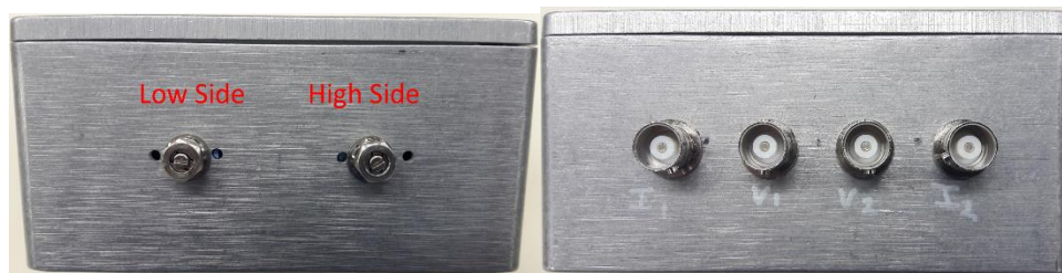
Figure 39: The enclosure for the two 500\text{ k}\Omega potentiometers that are used for tuning the voltage divider ratio.
